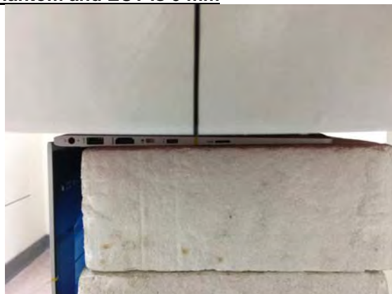
Fig.6 EUT Laptop mode to flat phantom
