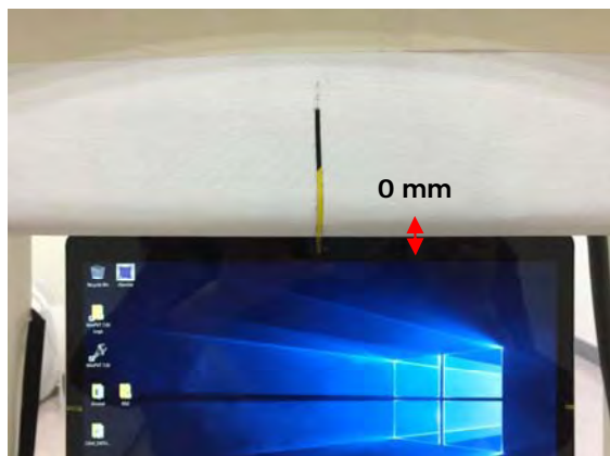
Fig.5 EUT Top side to flat phantom
