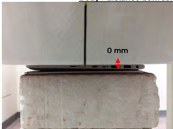
Fig.3 EUT Back side to flat phantom
