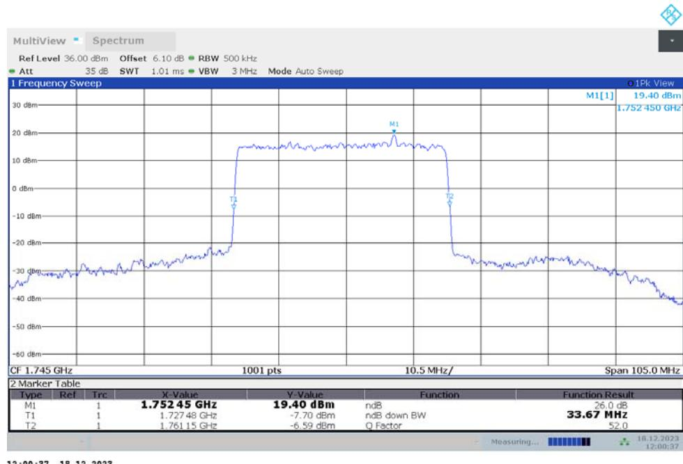
**n66,35MHz Bandwidth,DFT-s-QPSK (-26dBc BW)**
