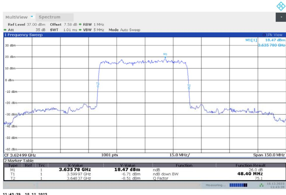
**n48,50MHz Bandwidth,DFT-s-QPSK (-26dBc BW)**
