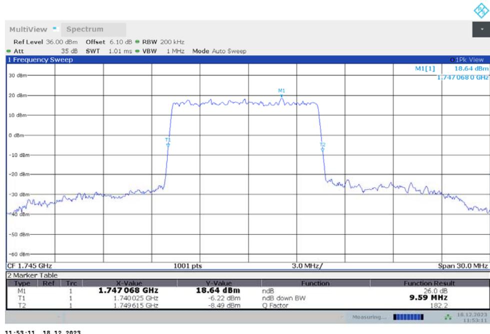
**n66,10MHz Bandwidth,DFT-s-QPSK (-26dBc BW)**
