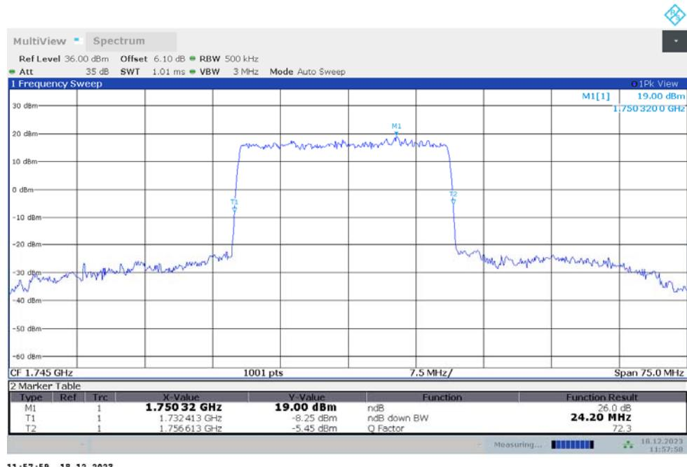
**n66,25MHz Bandwidth,DFT-s-QPSK (-26dBc BW)**
