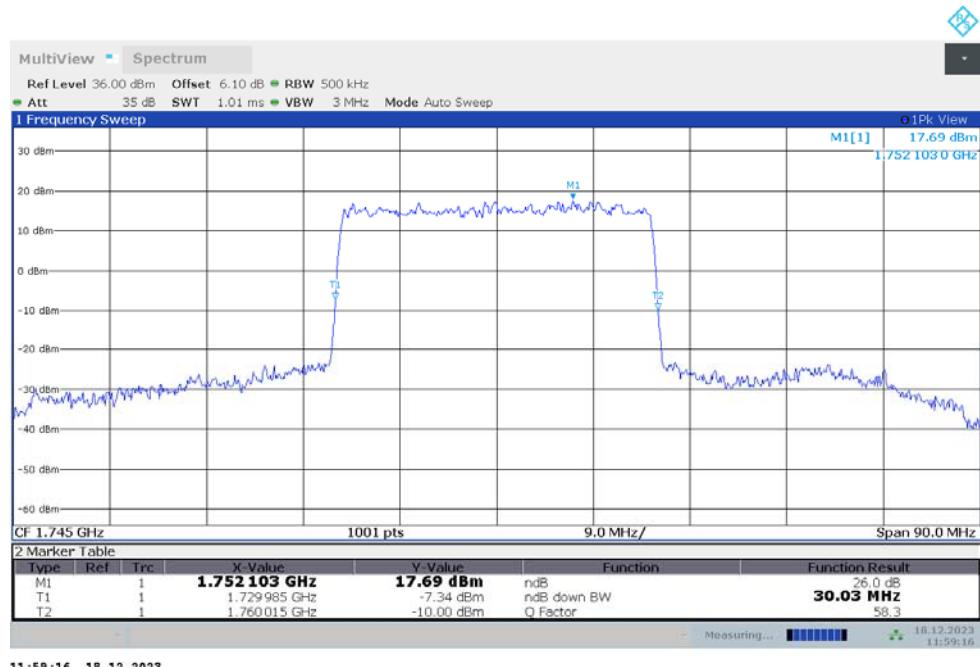
**n66,30MHz Bandwidth,DFT-s-QPSK (-26dBc BW)**
