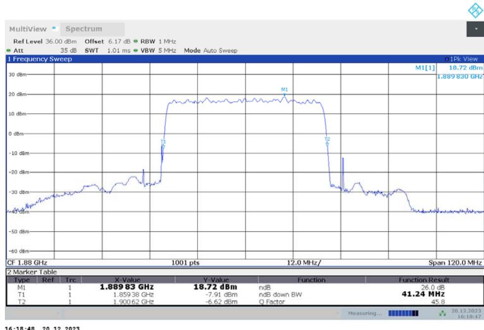
**n2,40MHz Bandwidth,DFT-s-QPSK (-26dBc BW)**
