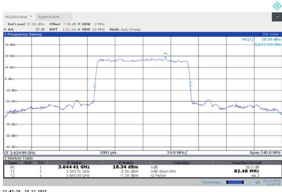
**n48,80MHz Bandwidth,DFT-s-QPSK (-26dBc BW)**
