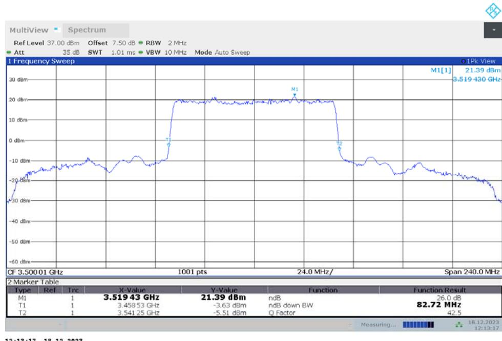
**n77L,80MHz Bandwidth,DFT-s-QPSK (-26dBc BW)**
