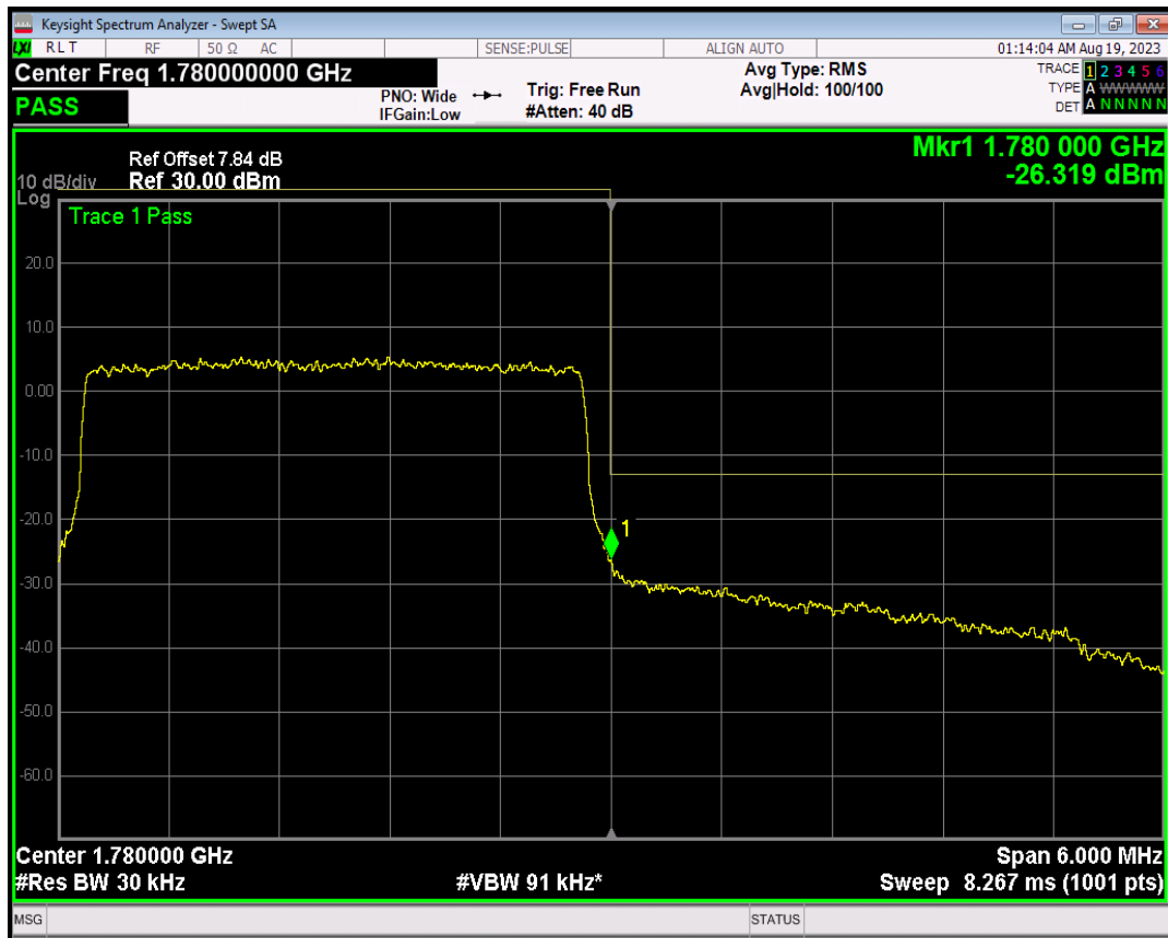
Band66 16QAM BW=3MHz Channel=132657 RB Size=1 Position=#0
