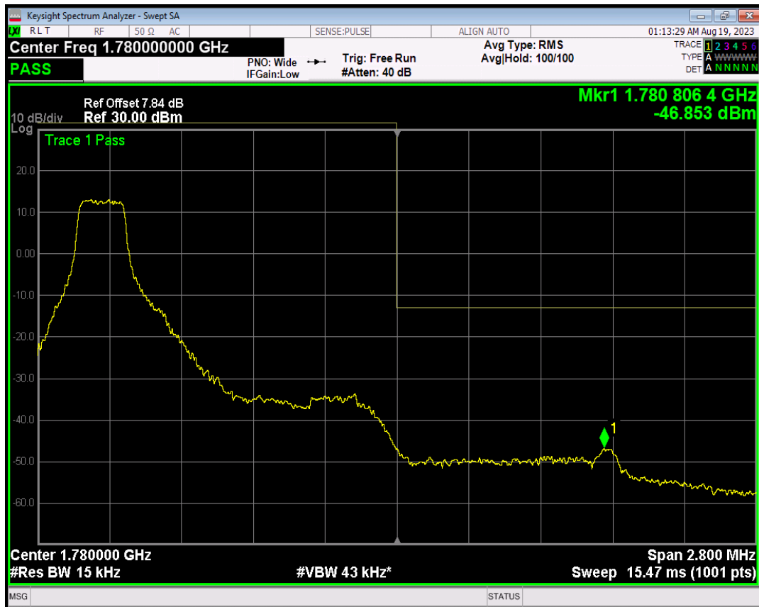
Band66 16QAM BW=1.4MHz Channel=132665 RB Size=1 Position=#Max
