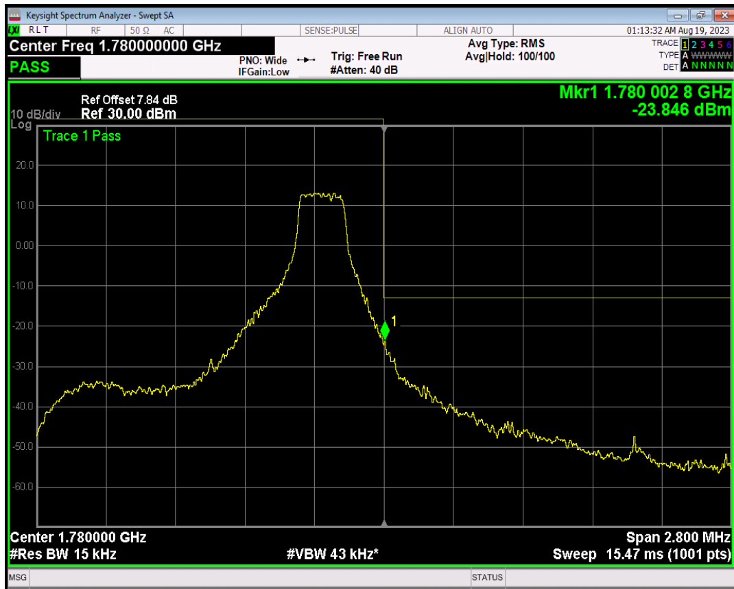
Band66 16QAM BW=1.4MHz Channel=132665 RB Size=6 Position=#0
