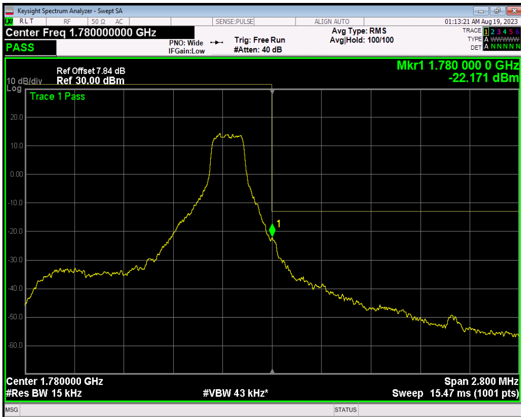
Band66 QPSK BW=1.4MHz Channel=132665 RB Size=6 Position=#0
