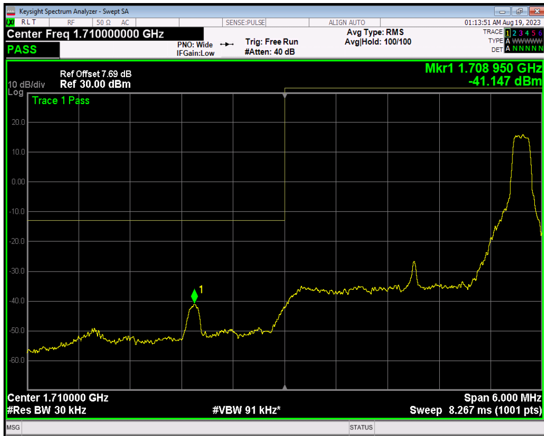
Band66 16QAM BW=3MHz Channel=131987 RB Size=15 Position=#0
