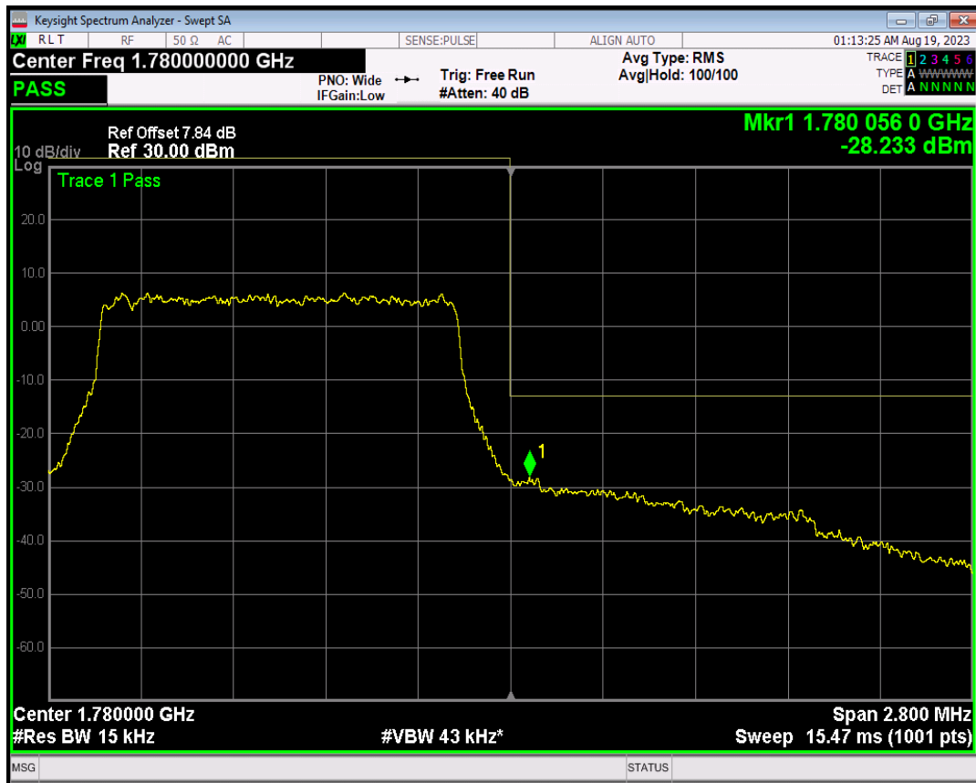
Band66 16QAM BW=1.4MHz Channel=132665 RB Size=1 Position=#0
