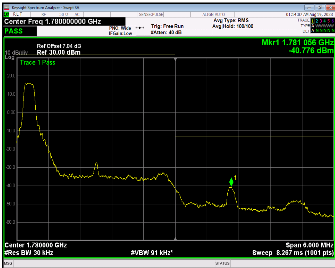
Band66 16QAM BW=3MHz Channel=132657 RB Size=1 Position=#Max
