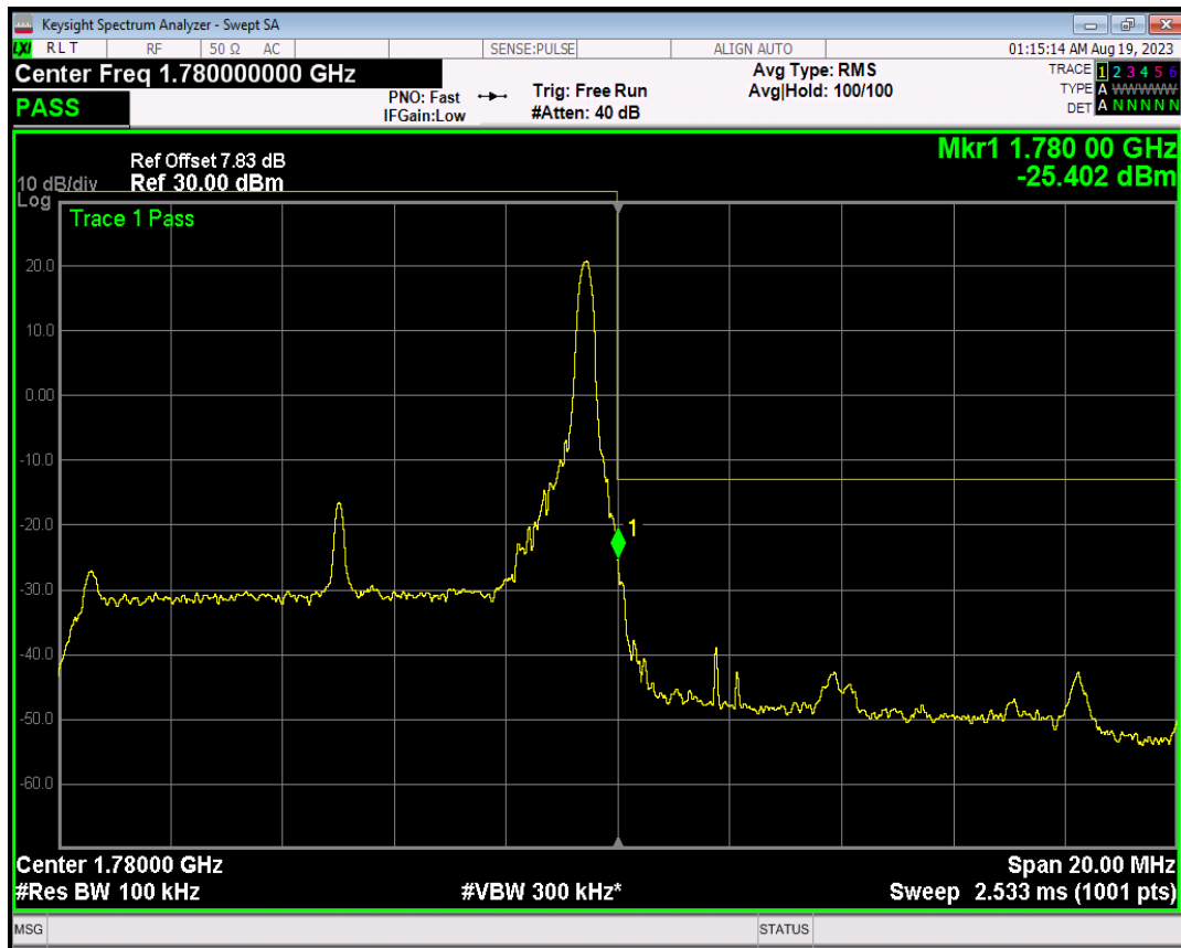
Band66 16QAM BW=10MHz Channel=132622 RB Size=50 Position=#0
