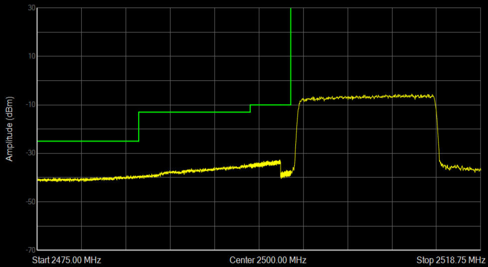
Band7 16QAM BW=15MHz Channel=20825 RB Size=75 Position=#0
