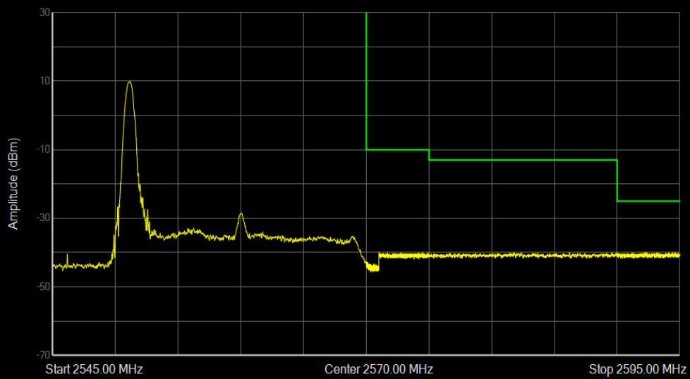
Band7 16QAM BW=20MHz Channel=21350 RB Size=1 Position=#0
