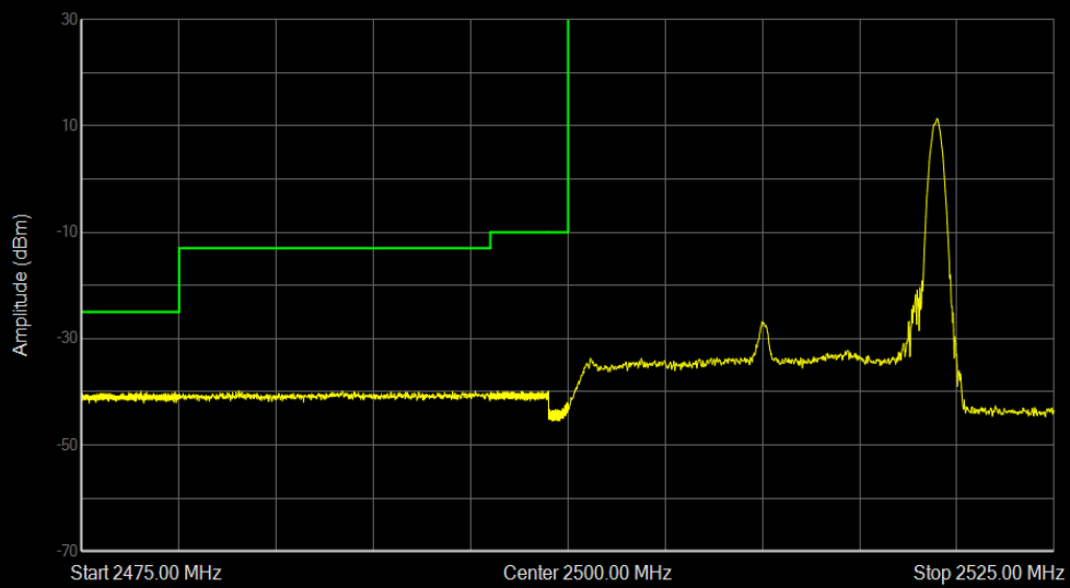
Band7 QPSK BW=20MHz Channel=20850 RB Size=1 Position=#Max
