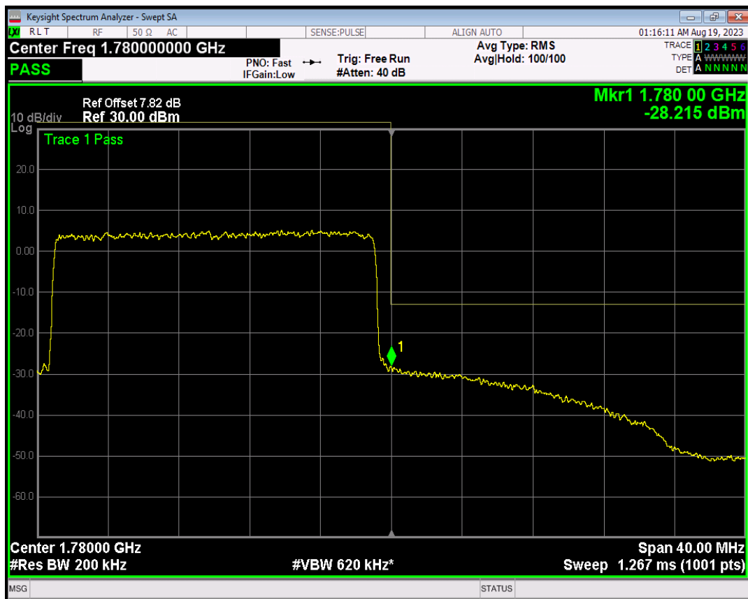
Band66 16QAM BW=20MHz Channel=132572 RB Size=1 Position=#Max
