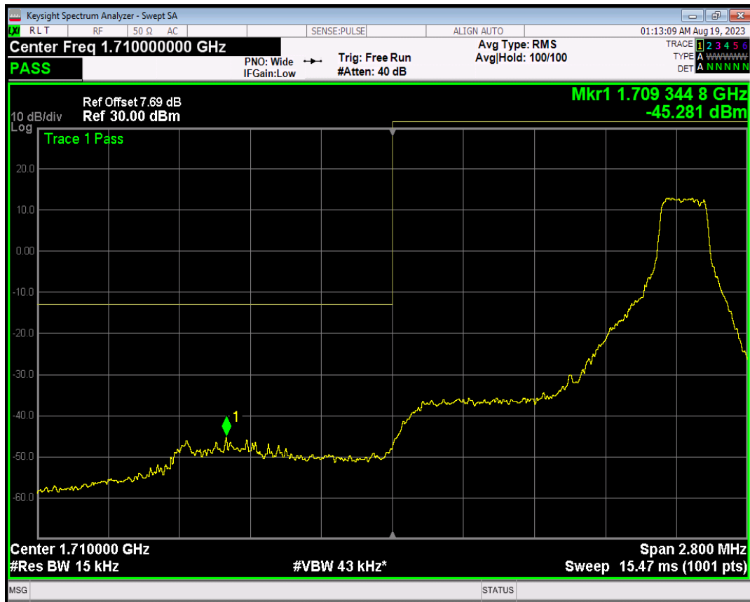
Band66 16QAM BW=1.4MHz Channel=131979 RB Size=6 Position=#0
