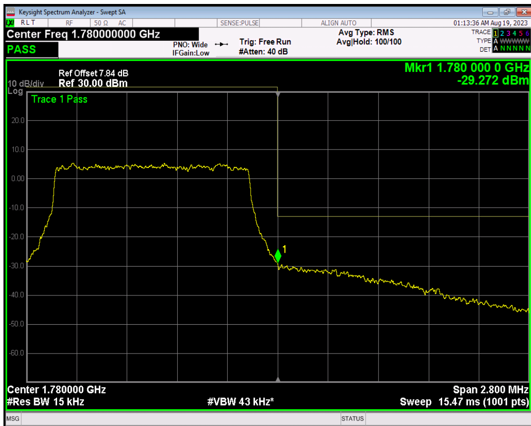
Band66 QPSK BW=3MHz Channel=131987 RB Size=1 Position=#0
