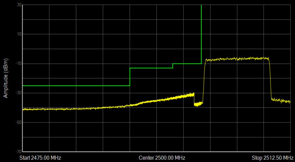
Band7 16QAM BW=10MHz Channel=20800 RB Size=50 Position=#0
