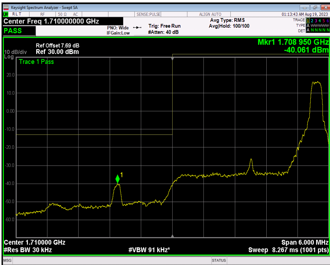
Band66 QPSK BW=3MHz Channel=131987 RB Size=15 Position=#0
