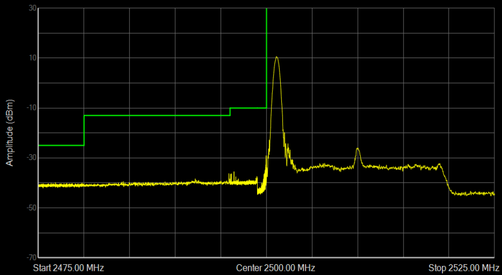
Band7 16QAM BW=20MHz Channel=20850 RB Size=1 Position=#0
