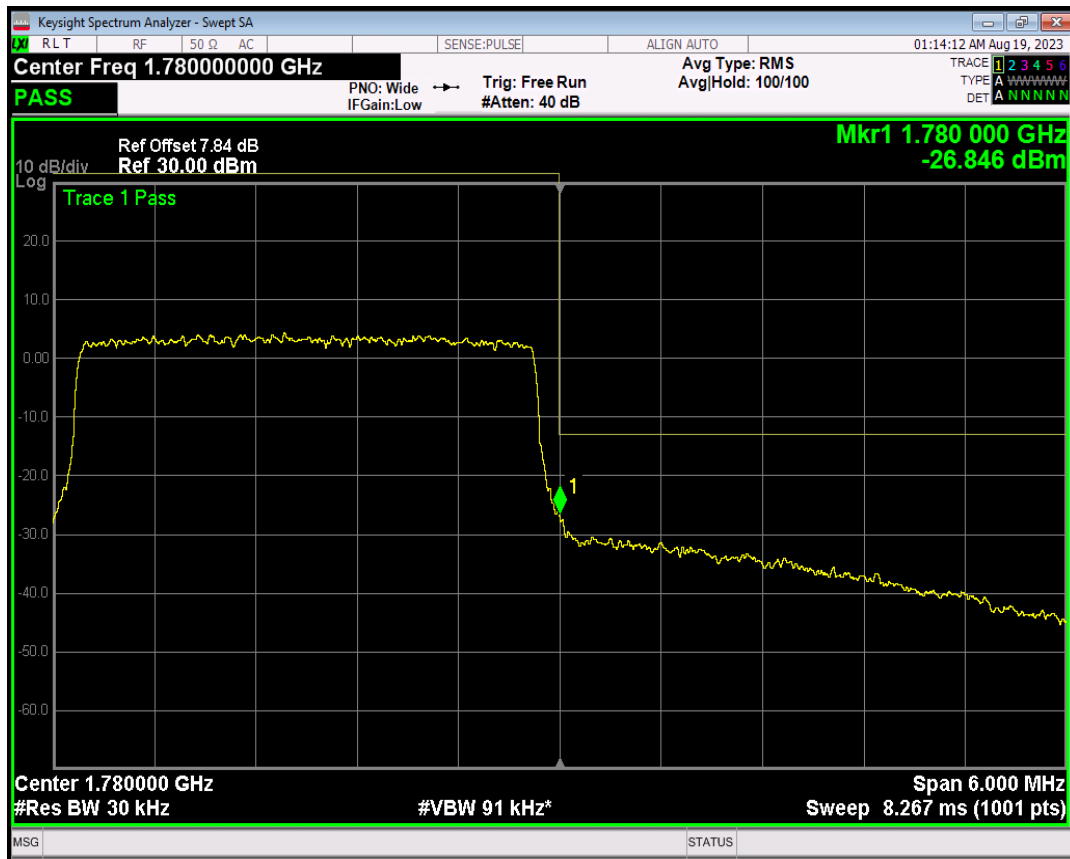
Band66 QPSK BW=5MHz Channel=131997 RB Size=1 Position=#Max
