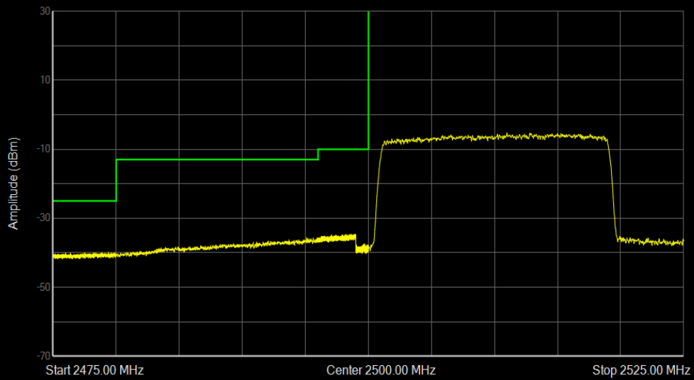
Band7 16QAM BW=20MHz Channel=20850 RB Size=100 Position=#0
