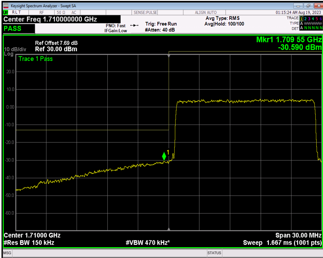
Band66 16QAM BW=15MHz Channel=132047 RB Size=1 Position=#0
