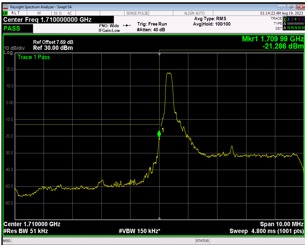
Band66 16QAM BW=5MHz Channel=131997 RB Size=1 Position=#Max
