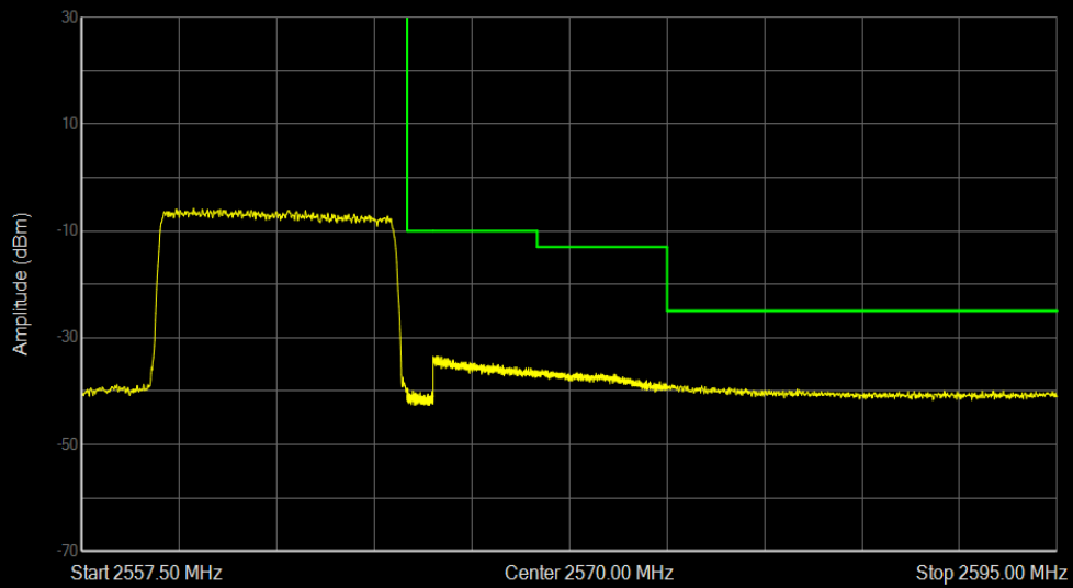
Band7 16QAM BW=10MHz Channel=21400 RB Size=50 Position=#0
