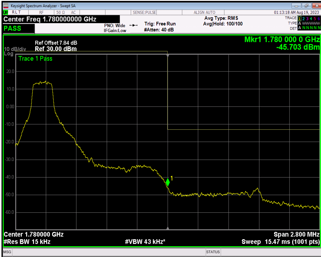
Band66 QPSK BW=1.4MHz Channel=132665 RB Size=1 Position=#Max
