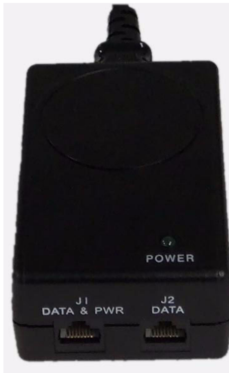
Figure 7 PoE Injector - Data & PWR and Data Ports
