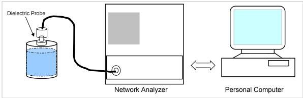
Set-up for liquid parameters check
