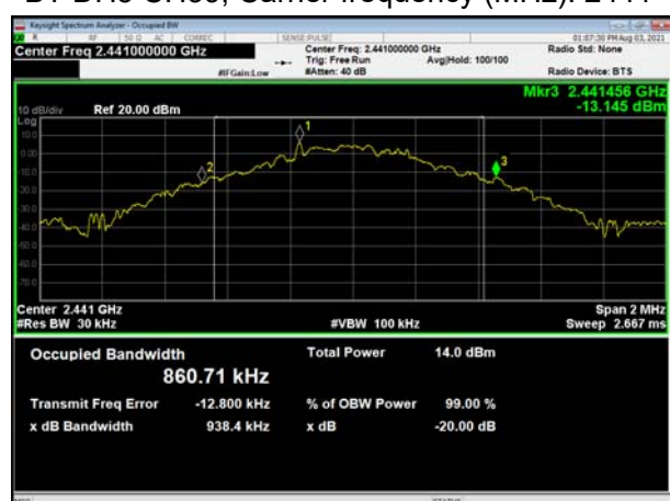
BT DH5 CH78, Carrier frequency (MHz): 2480
