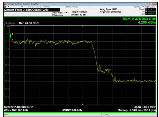
BT 3DH5 CH78, Carrier frequency (MHz): 2480
