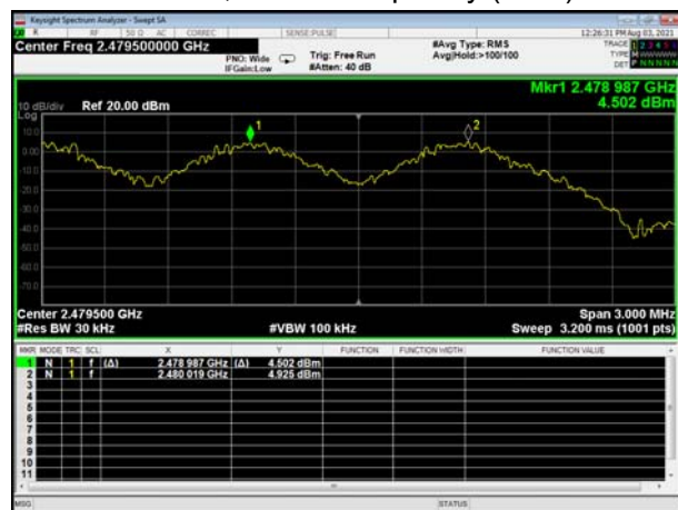
BT DH5 CH78, Carrier frequency (MHz): 2480
