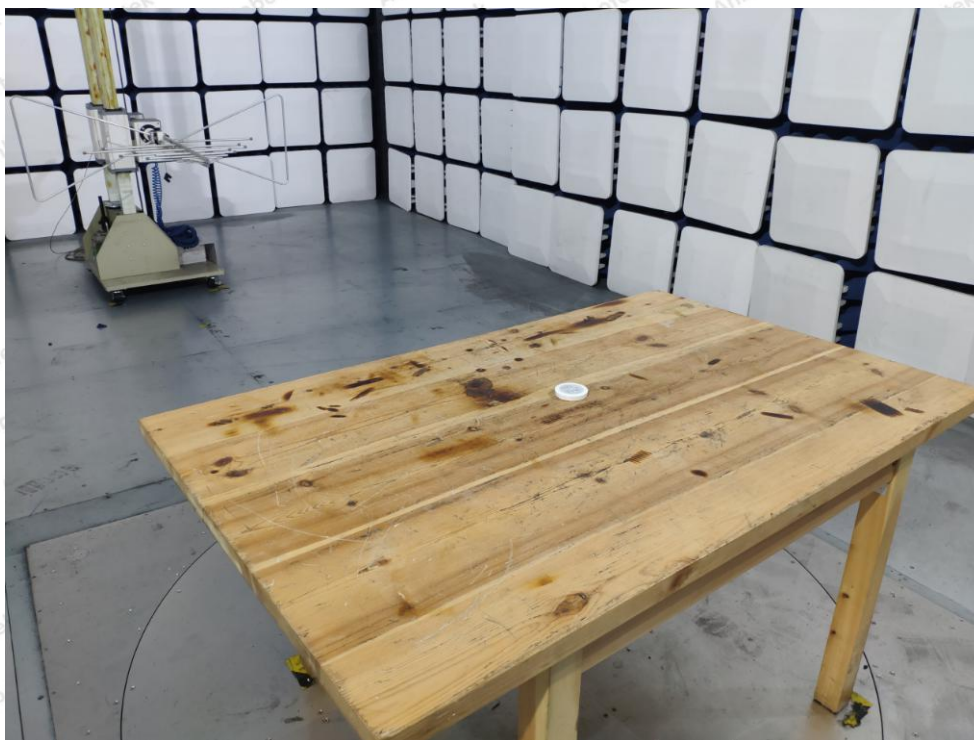
Photo of Radiation Emission Test
