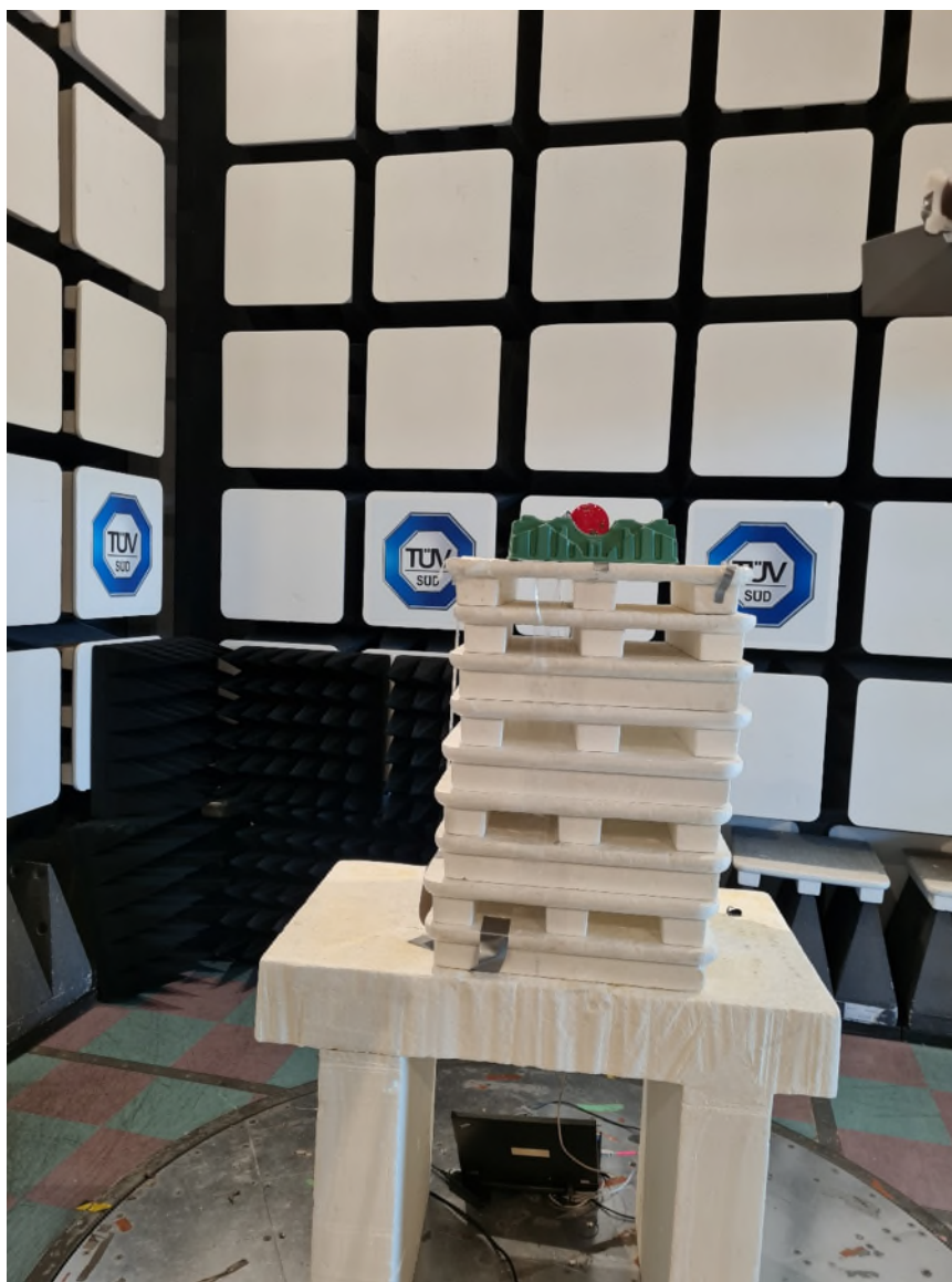
Figure 6 – Radiated Emissions Setup
