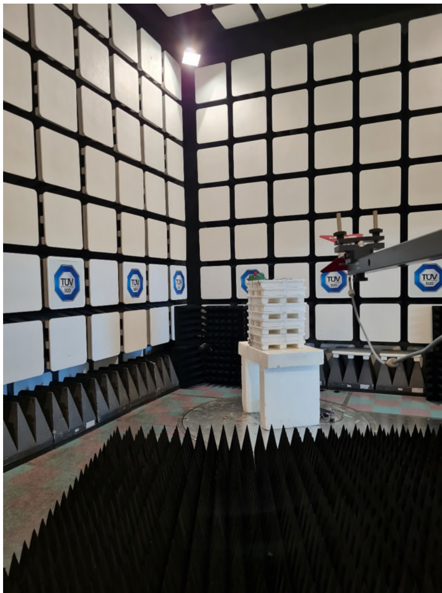
Figure 4 – Radiated Emissions Setup
