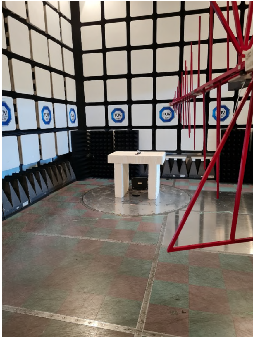
Figure 3 – Radiated Emissions Setup
