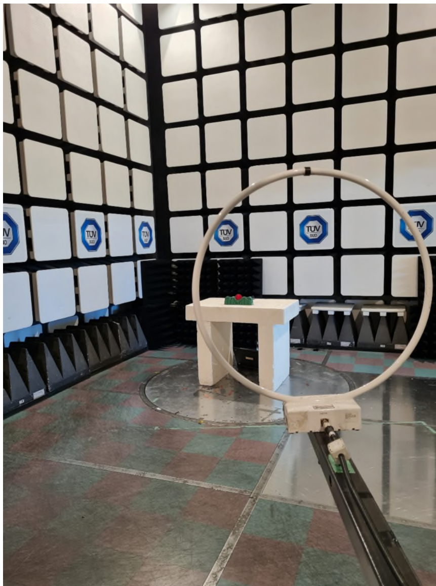
Figure 2 – Radiated Emissions Setup
