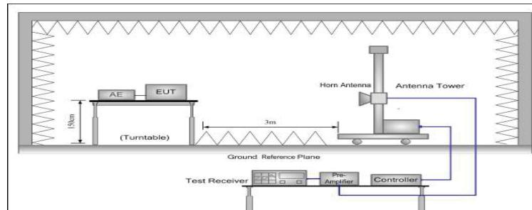
1. The EUT was placed on the top of a rotating table 0.8 meters above the ground at a 3 meter camber. The table was rotated 360 degrees to determine the position of the highest radiation.
