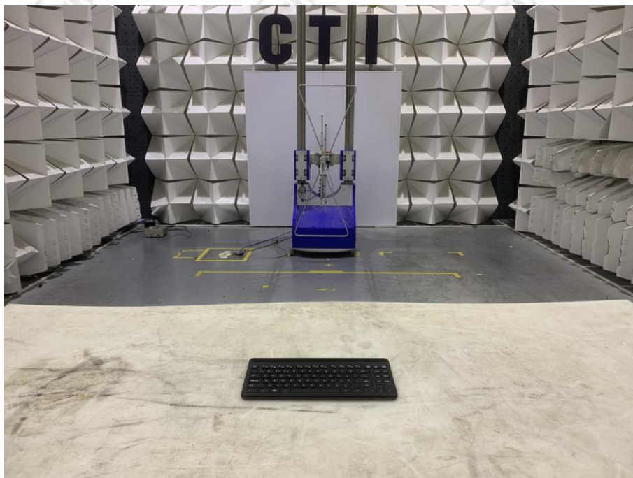
Radiated spurious emission Test Setup-1(Below 1GHz)
