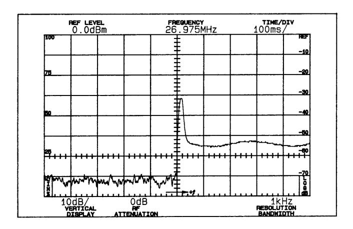
Measurement Conditions: 16 dB over 50% modulation level at 1200 Hz with 2500 Hz tone, upper fourth order sideband; horizontal scale 100 ms/div.
