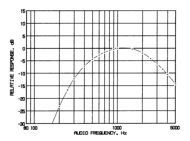
TRANSMITTER FREQUENCY RESPONSE FCC ID: MMA77235ESP
