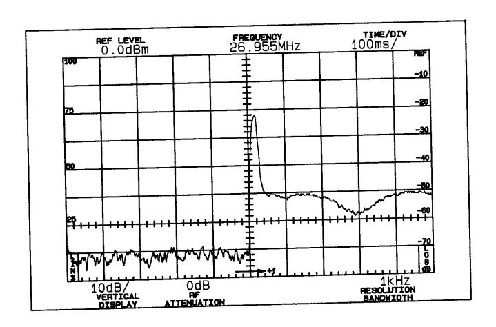
Measurement Conditions: 16 dB over 50% modulation level at 1200 Hz with 2500 Hz tone, lower fourth order sideband; horizontal scale 100 ms/div.
