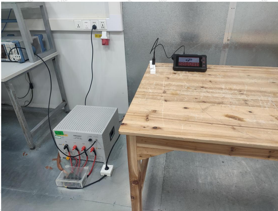
Photo of Power Line Conducted Emission Test
