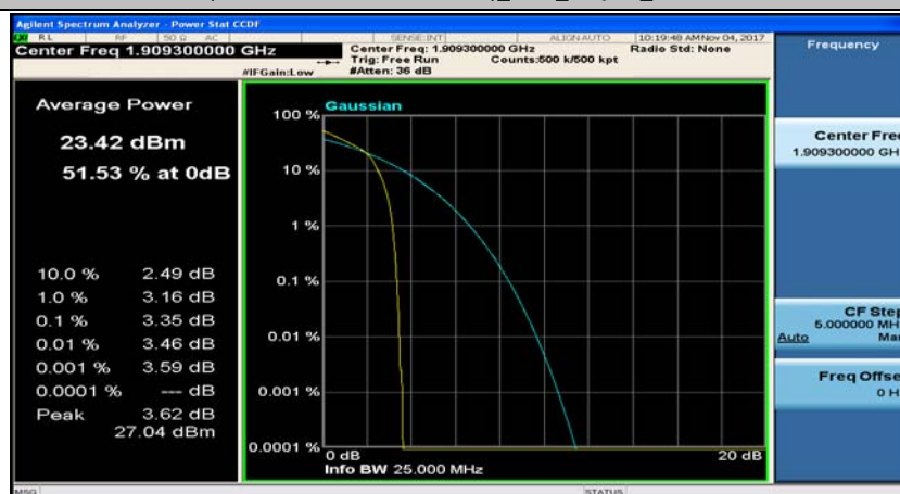
(Channel Bandwidth: 1.4 MHz)_HCH_16QAM_3RB#2
