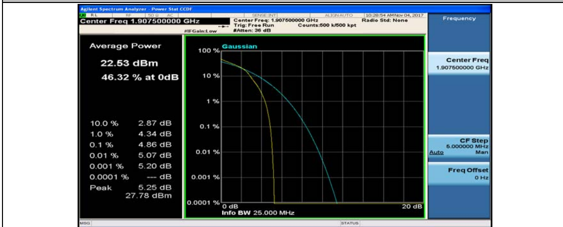
(Channel Bandwidth: 5 MHz)_HCH_16QAM_25RB#0
