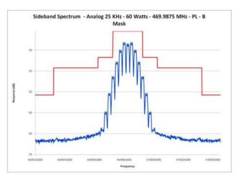
E1-5.23 Occupied Bandwidth, Analog, 25 kHz Channels, 469.9875 MHz PL
