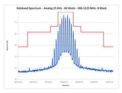
E1-5.7 Occupied Bandwidth, Analog, 25 kHz Channels, 406.1125 MHz
