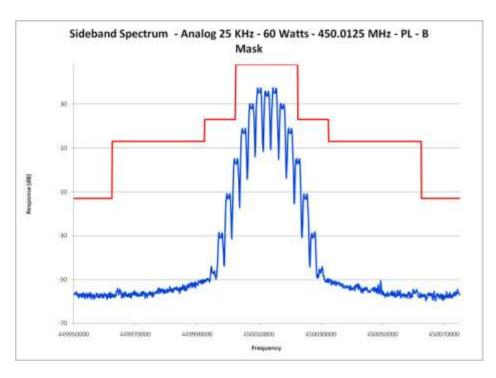
E1-5.17 Occupied Bandwidth, Analog, 25 kHz Channels, 450.0125 MHz PL
