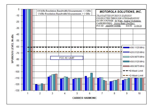
E1-6.1 Conducted Spurious Harmonic Emissions, Power Output 60 Watts
