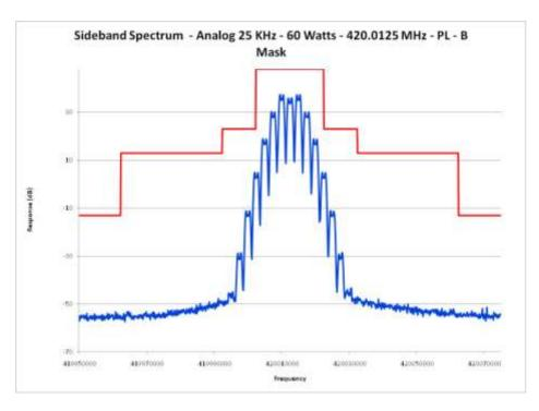
E1-5.11 Occupied Bandwidth, Analog, 25 kHz Channels, 420.0125 MHz PL
