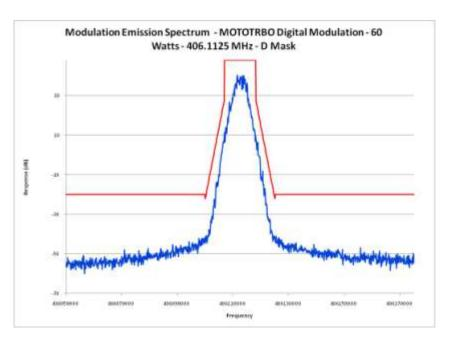
E1-5.1 Occupied Bandwidth – MOTOTRBO<sup>™</sup> Digital Modulation, 406.1125 MHz
