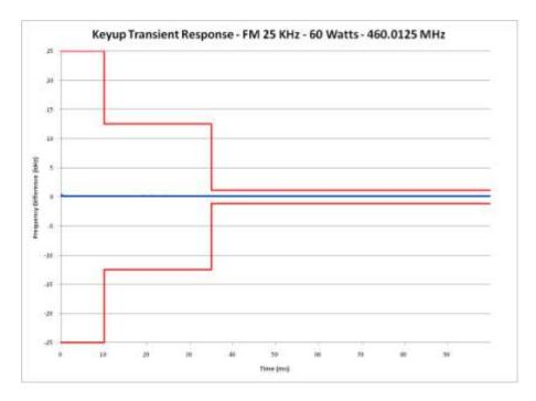
E1-9.1 Frequency Transient Behavior, 25 kHz Channel Key-Up, 460.0125MHz
