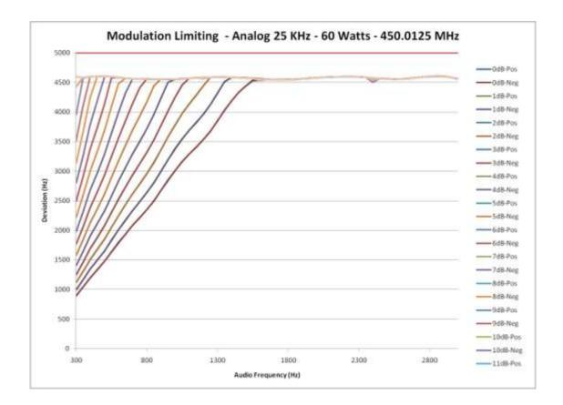
E1-11.5 Audio Modulation Limiting – Modulation Characteristics, 25 kHz Channels – 460.0125 MHz
