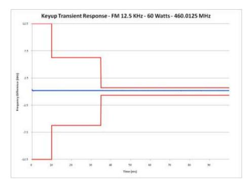
E1-9.3 Frequency Transient Behavior, 12.5 kHz Channel Key-Up, 460.0125 MHz
