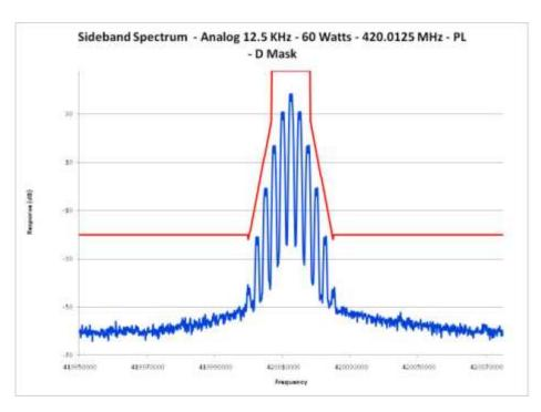
E1-5.29 Occupied Bandwidth, Analog, 12.5 kHz Channels, 420.0125 MHz PL
