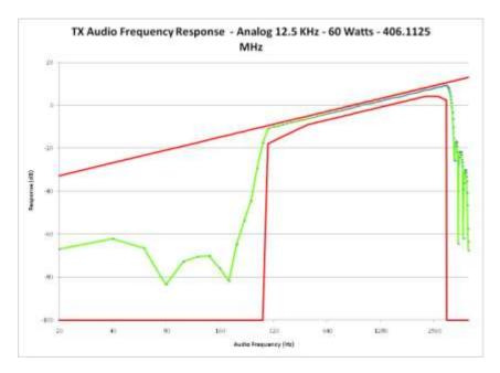
E1-10.8 Audio Frequency Response – Modulation Characteristics, 12.5 kHz Channels – 420.0125 MHz
