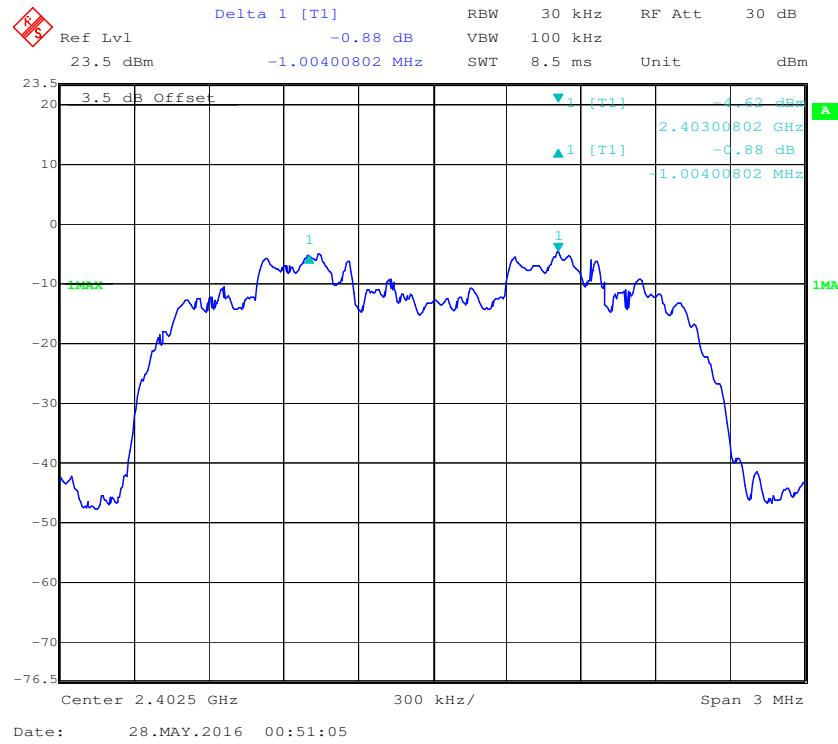
**EDR ( $\pi/4$ -DQPSK): Middle Channel**
