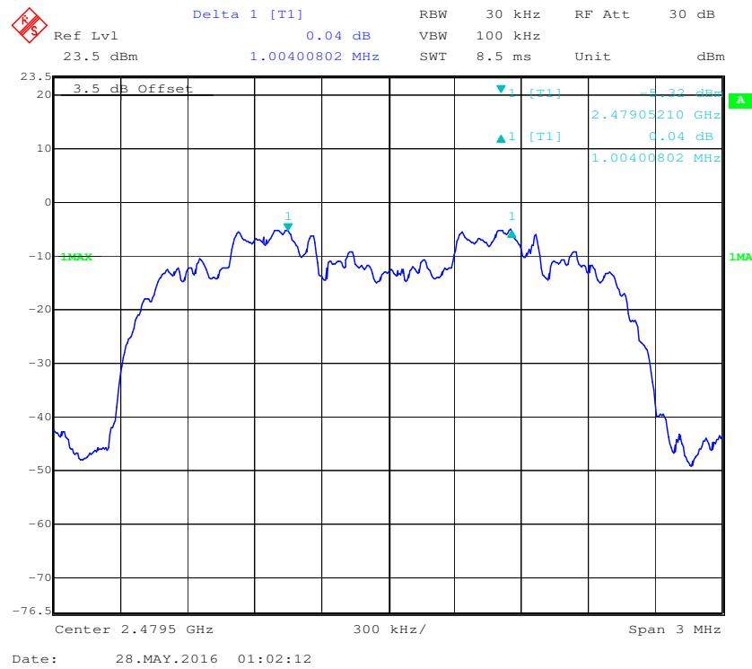
**EDR (8DPSK): Low Channel**
