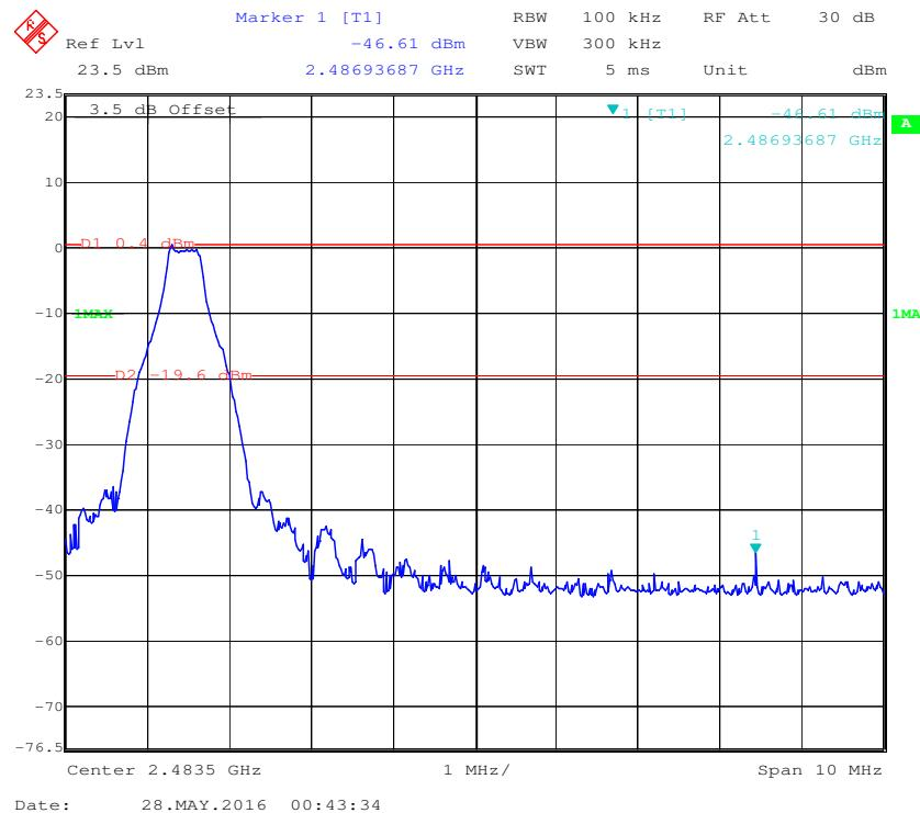
**EDR ( $\pi/4$ -DQPSK): Band Edge-Left Side**
