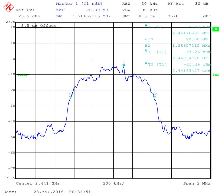
**EDR ( $\pi/4$ -DQPSK): High Channel**
