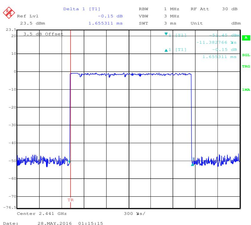
**Pulse time, High Channel, 2DH3**
