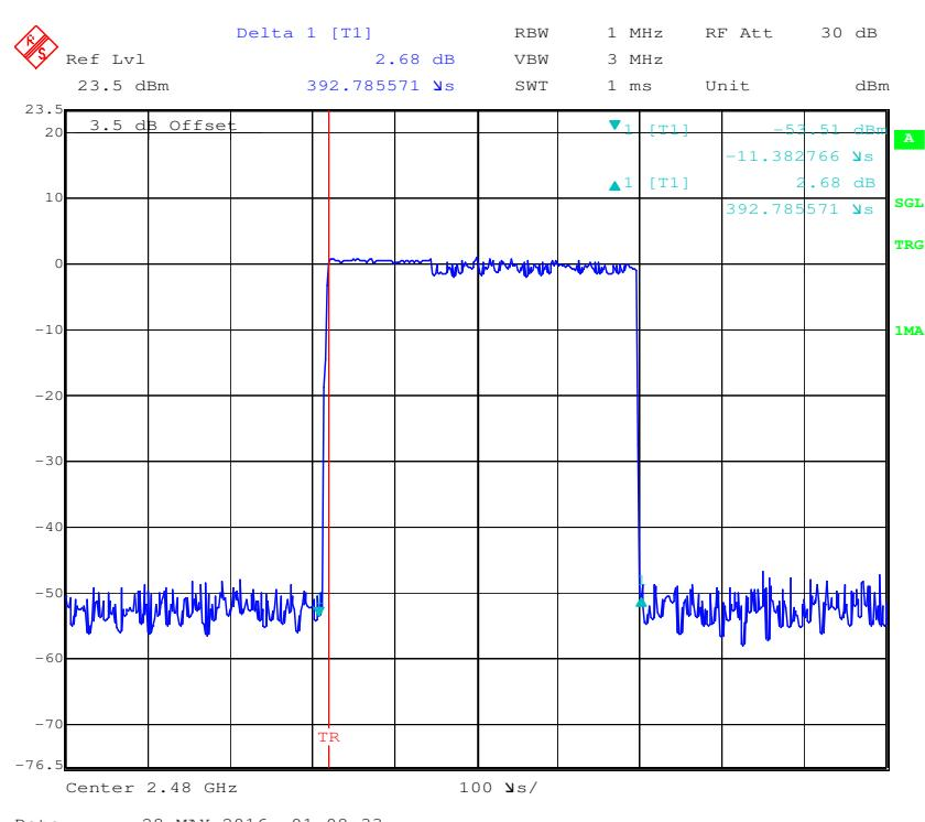
**Pulse time, Low Channel, 2DH3**
