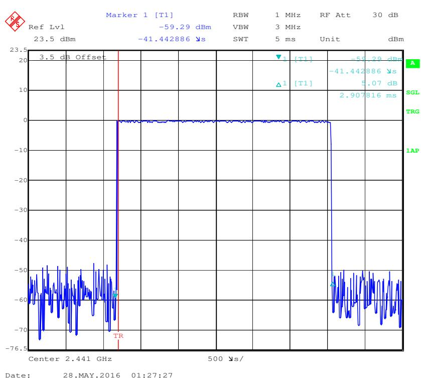
**Pulse time, High Channel, DH5**
