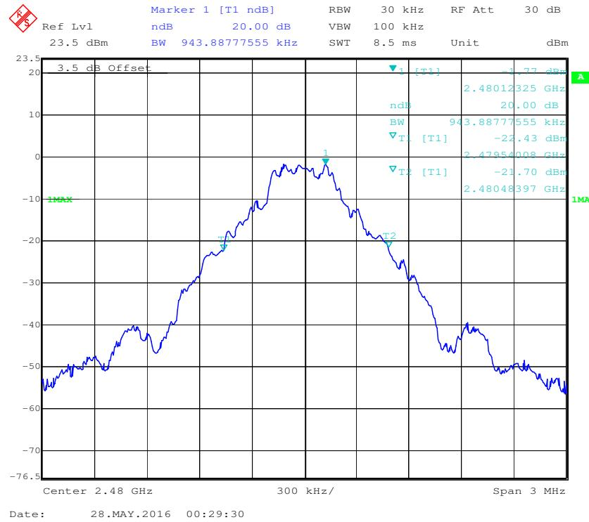
**EDR ( $\pi/4$ -DQPSK): Low Channel**
