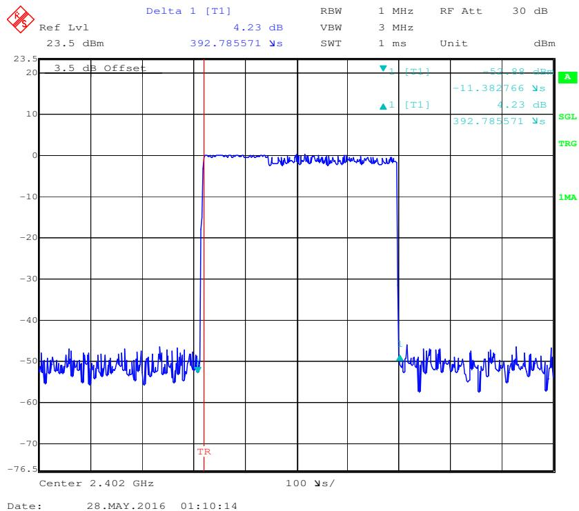
**Pulse time, Middle Channel, 2DH1**
