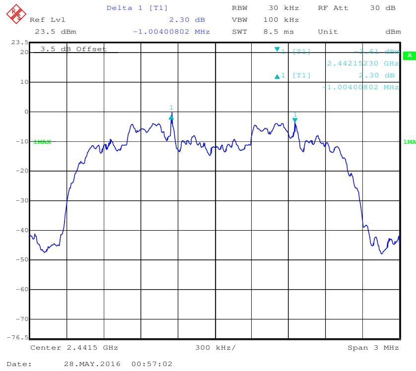
**EDR ( $\pi/4$ -DQPSK): High Channel**
