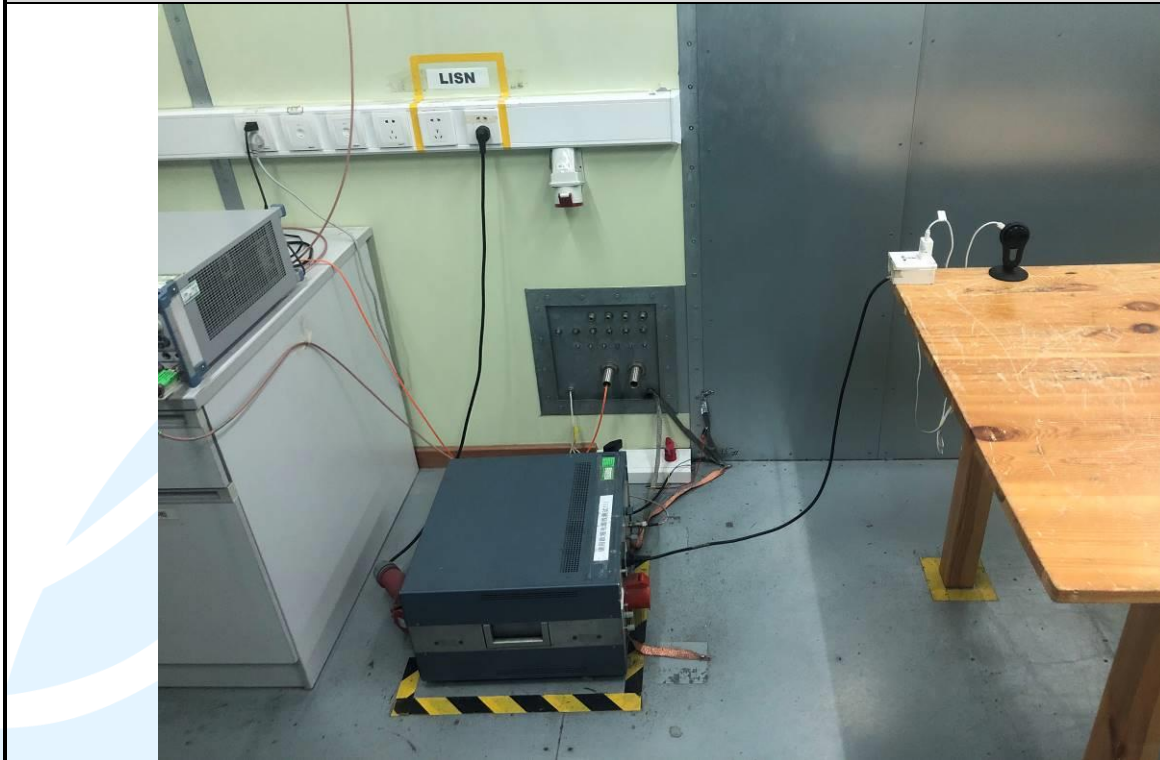
Conducted Emission Test Setup
