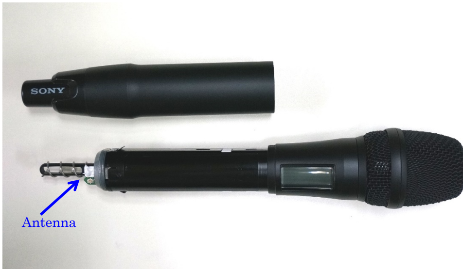
Fig.1: Removed the Grip (Place of Antenna)
