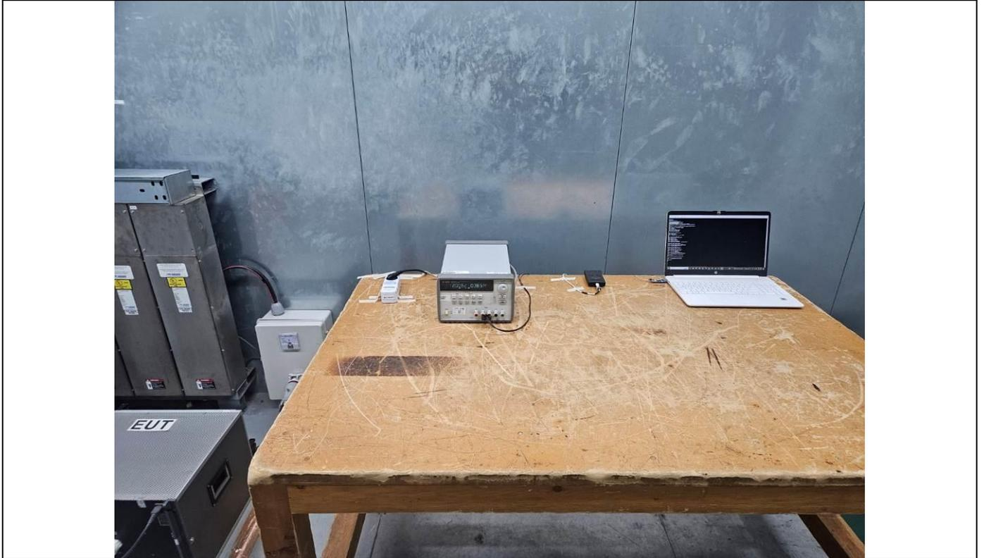
**- Radiated Emission Test (Below 1 GHz)**
