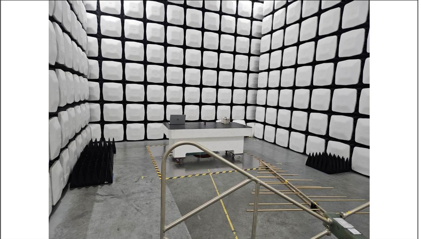
**- Radiated Emission Test (Above 1 GHz)**
