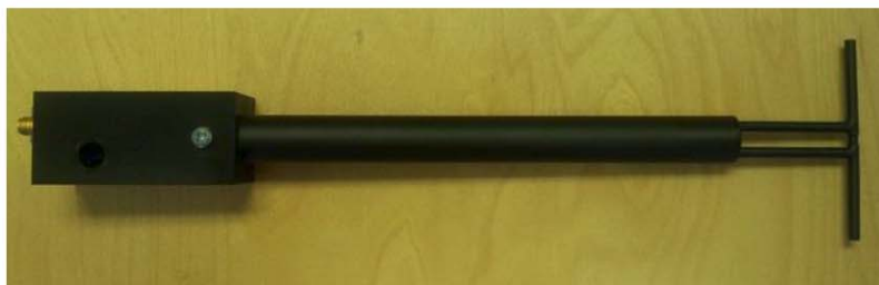
Figure 1 – MVG COMOSAR Validation Dipole
