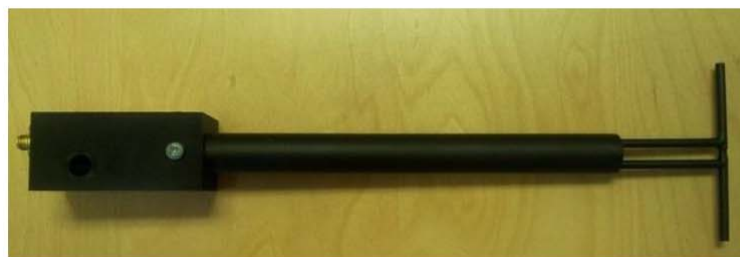
Figure 1 – MVG COMOSAR Validation Dipole
