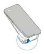
2. Install the nano-SIM card and the microSDXC card as shown
