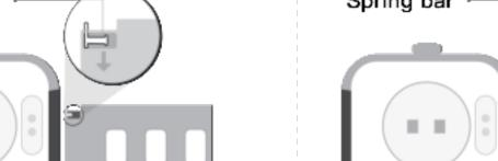
3. Press the band into the body and release the spring
