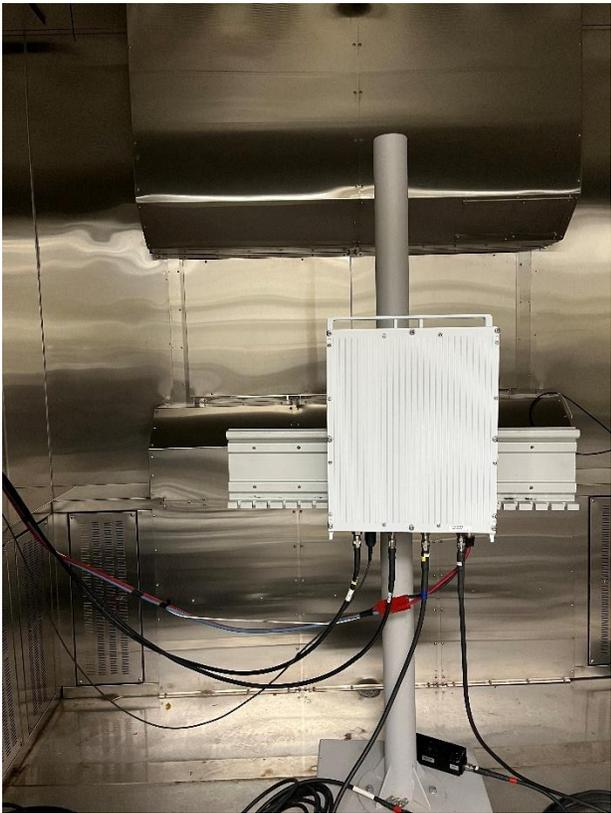
**Figure 3:** EUT Set-up photo for Thermal Radio Compliance Testing
