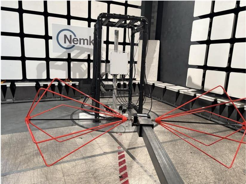
**Figure 4:** EUT Set-up photos for Radiated Emissions below 30 to 200 MHz
