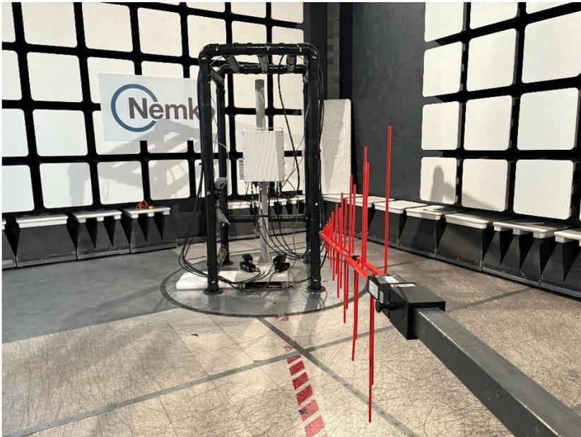
Figure 5: EUT Set-up photos for Radiated Emissions below 200 to 1000 MHz
