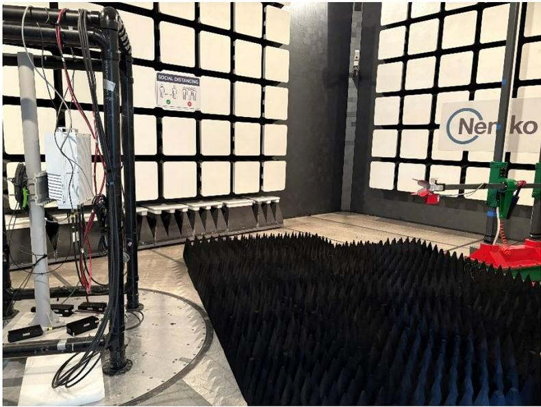
*Figure 7: EUT Set-up photos for Radiated Emissions above 1 GHz*
