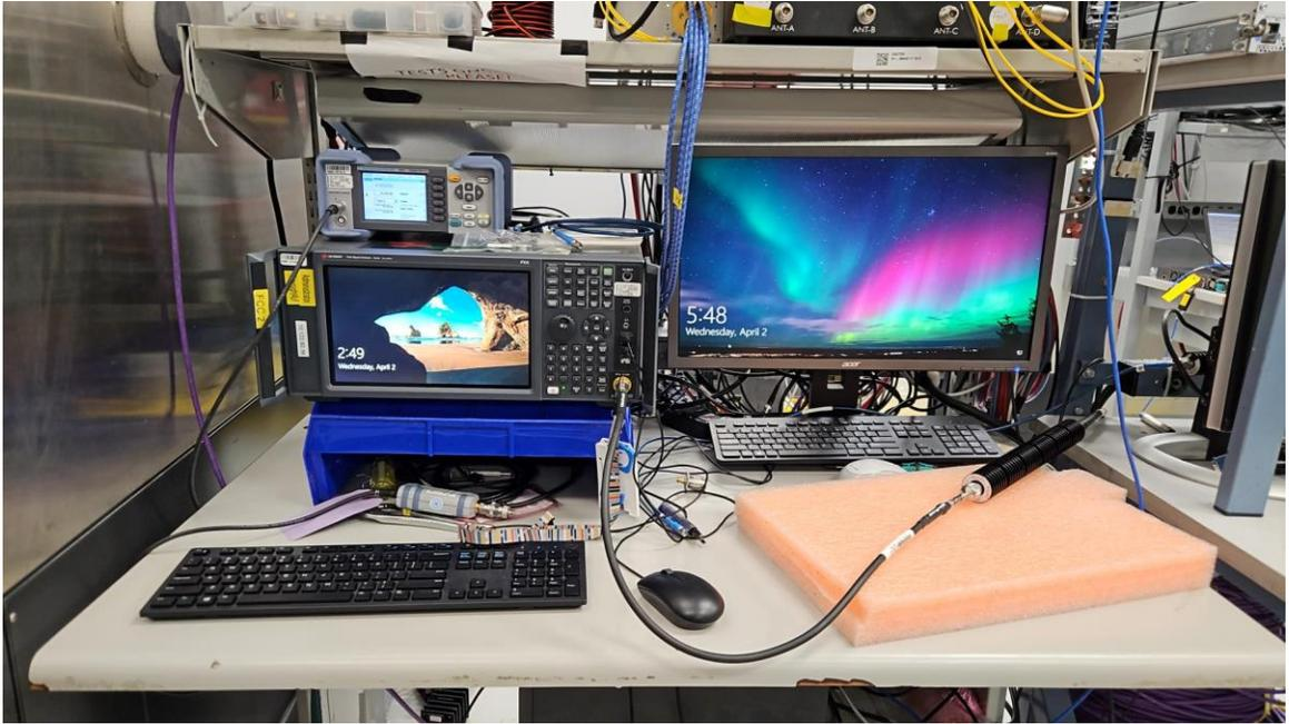
**Figure 1:** Set up photo for Radio Compliance Testing
