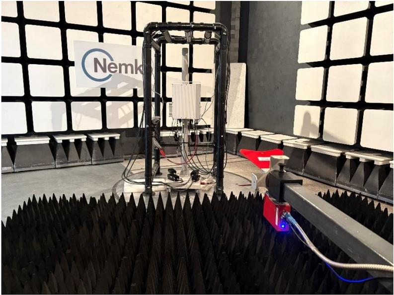
Figure 6: EUT Set-up photos for Radiated Emissions above 1 GHz
