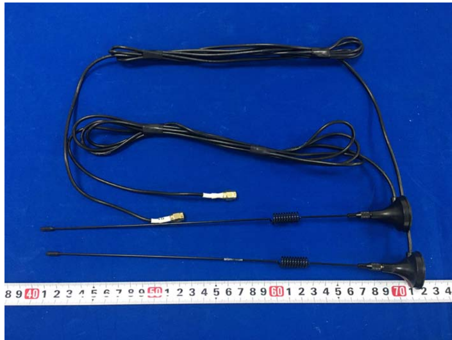
4G Antenna View
