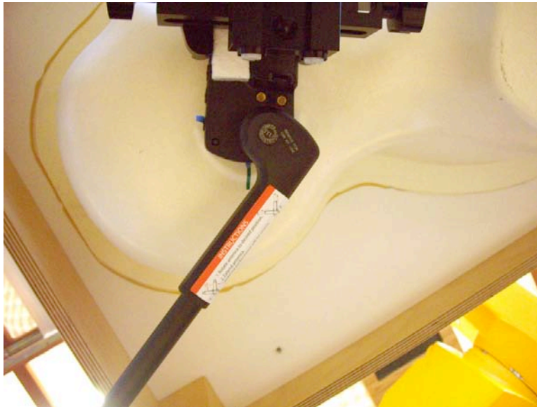
Figure 6-9 Phone positioned on Right phantom head, Antenna position 2
