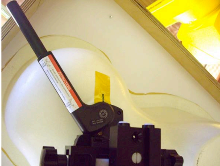
Figure 6-5 Phone positioned on Left phantom head, Antenna position 3
