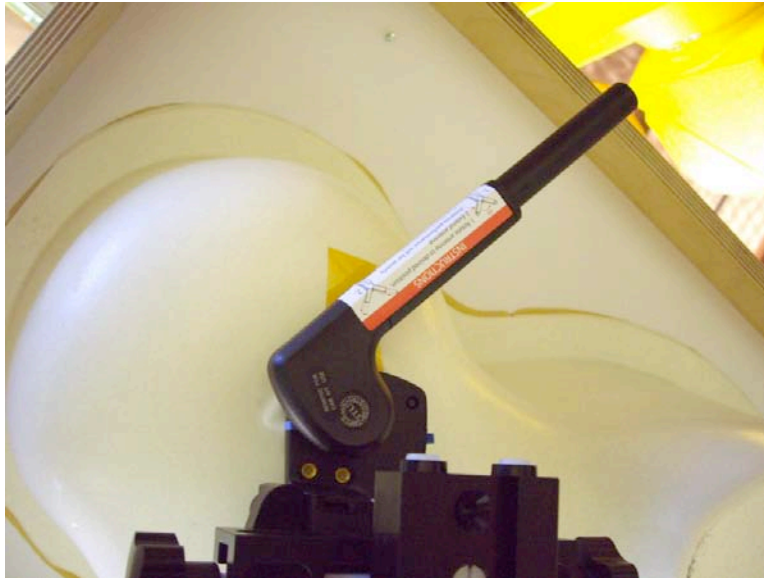
Figure 6-4 Phone positioned on Left phantom head, Antenna position 2
