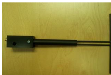
Figure 1 – MVG COMOSAR Validation Dipole
