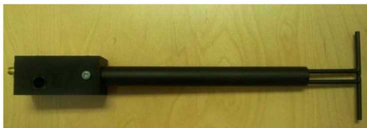
Figure 1 – MVG COMOSAR Validation Dipole
