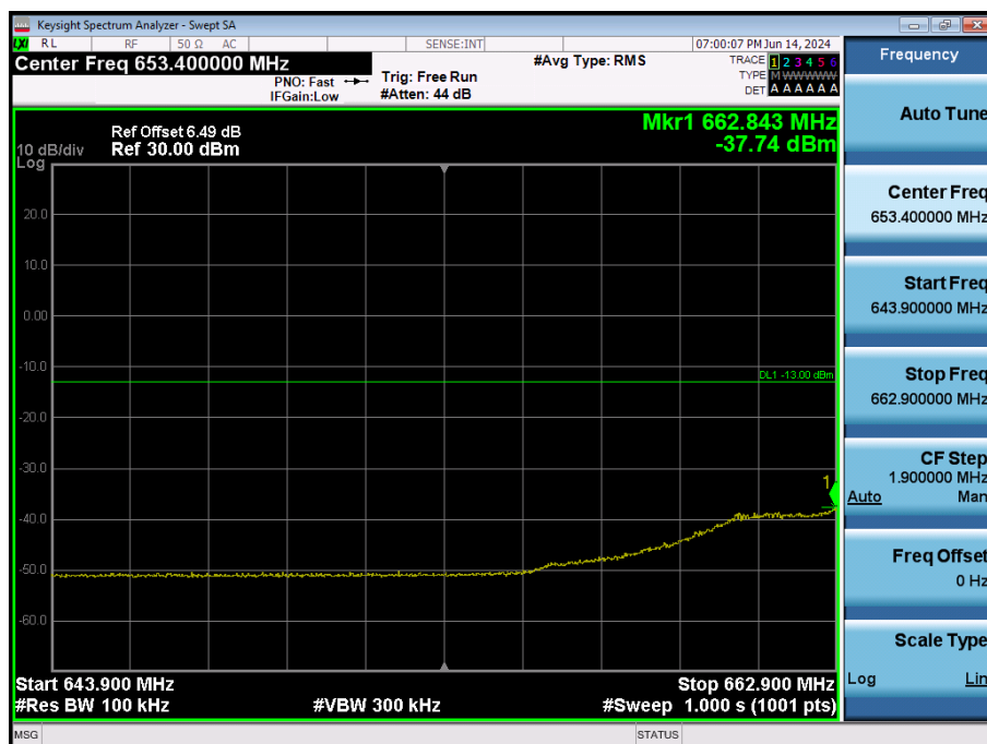
LTE Band 71 / 20MHz / QPSK - RB Size/Offset (100/0)
