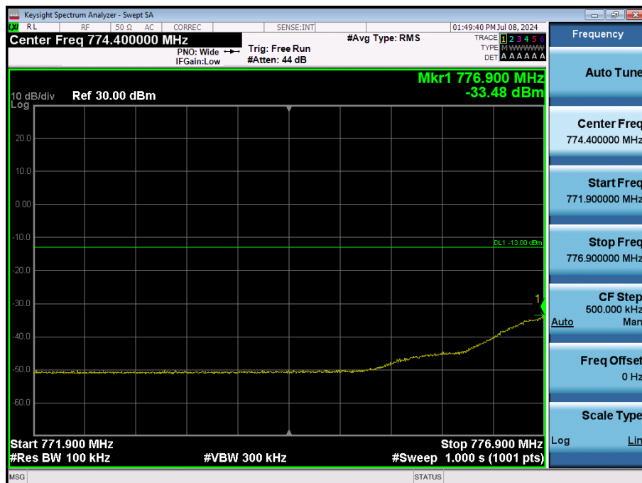
LTE Band 13 / 5MHz / 16QAM - RB Size/Offset (12/0)
