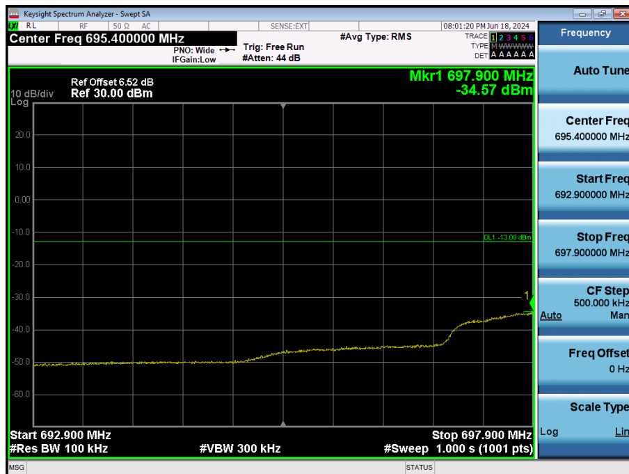
LTE Band 12 / 5MHz / QPSK - RB Size/Offset (12/0)
