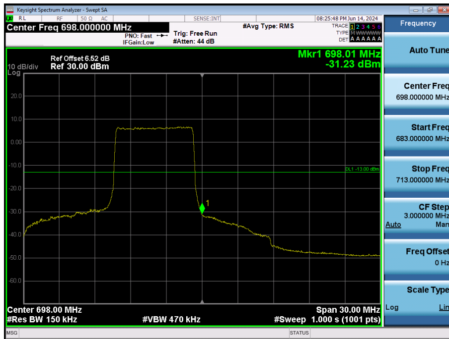
LTE Band 71 / 15MHz / QPSK - RB Size/Offset (36/39)
