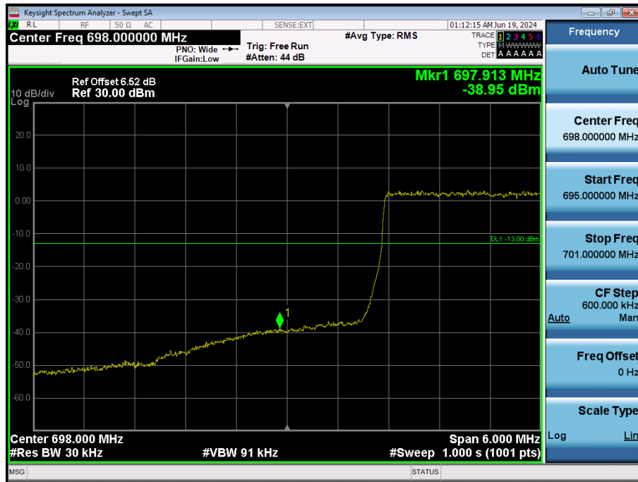
LTE Band 12 / 3MHz / 16QAM - RB Size/Offset (15/0)
