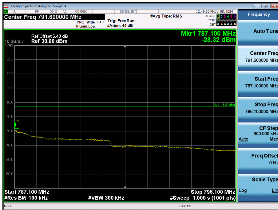
LTE Band 13 / 10MHz / QPSK - RB Size/Offset (25/25)
