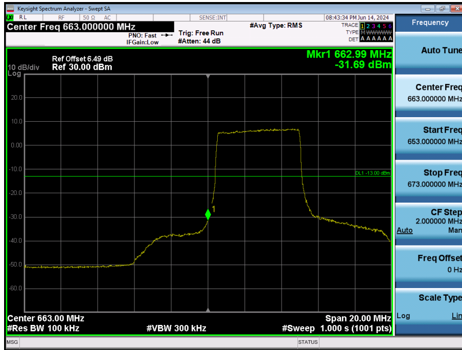
LTE Band 71 / 10MHz / QPSK - RB Size/Offset (25/0)
