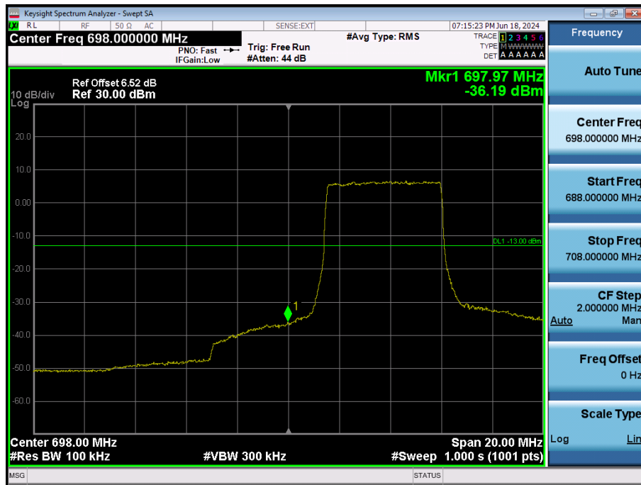
LTE Band 12 / 10MHz / QPSK - RB Size/Offset (25/0)
