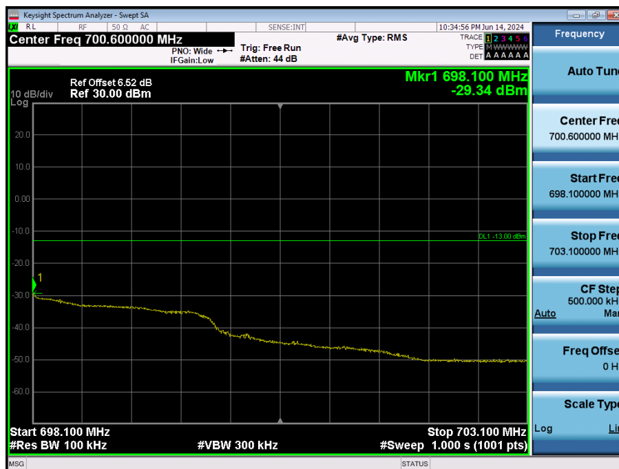
LTE Band 71 / 5MHz / QPSK - RB Size/Offset (12/13)
