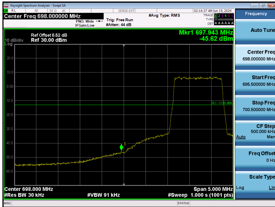
LTE Band 12 / 1.4MHz / 16QAM - RB Size/Offset (6/0)
