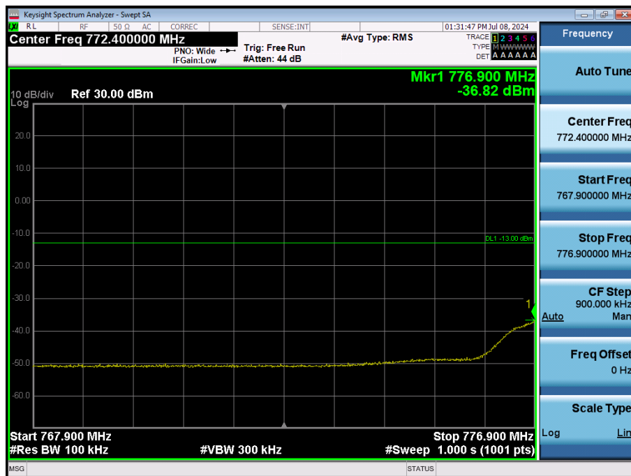
LTE Band 13 / 10MHz / 16QAM - RB Size/Offset (25/0)
