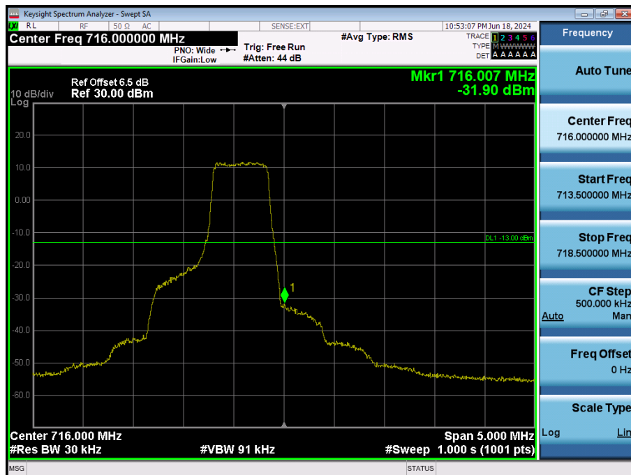
LTE Band 12 / 1.4MHz / QPSK - RB Size/Offset (3/3)
