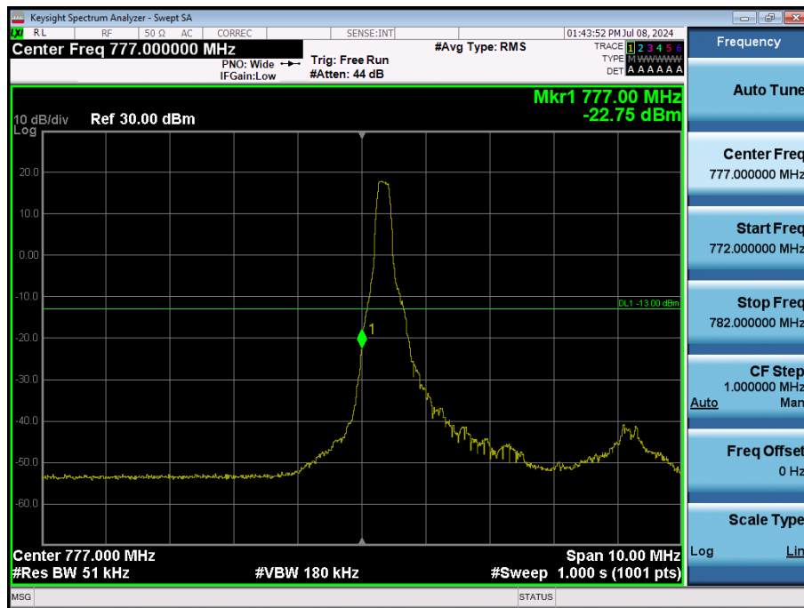
LTE Band 13 / 5MHz / 16QAM - RB Size/Offset (1/0)
