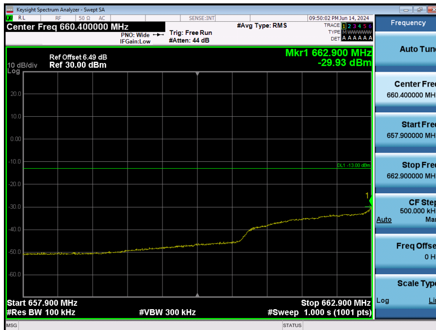
LTE Band 71 / 5MHz / QPSK - RB Size/Offset (12/0)
