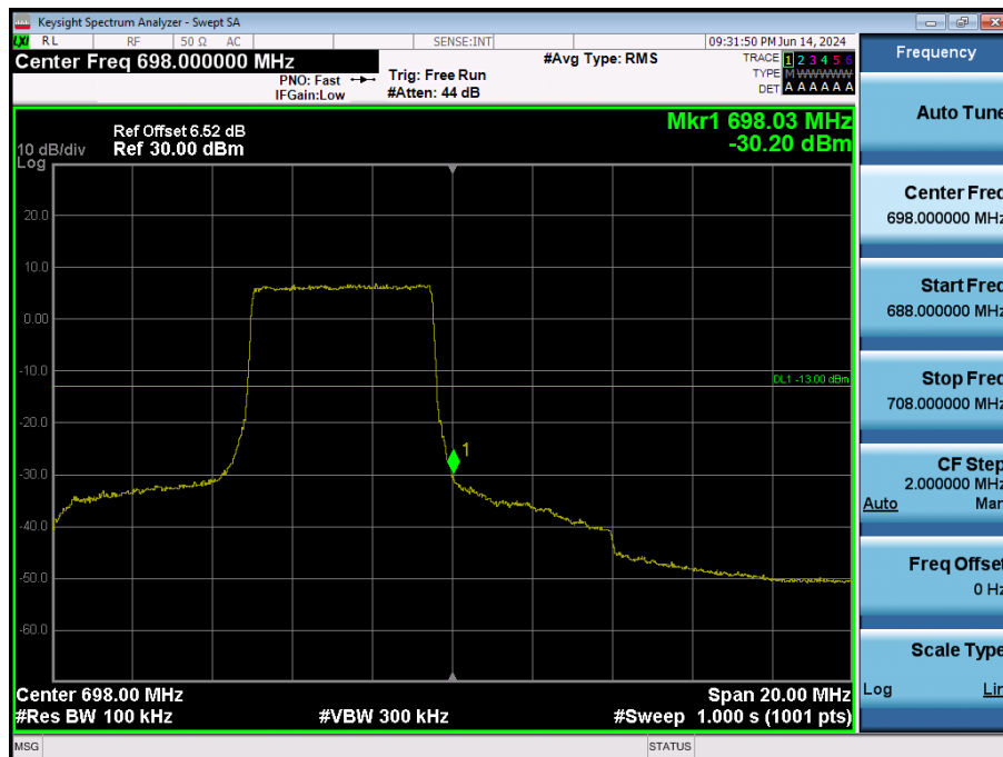
LTE Band 71 / 10MHz / QPSK - RB Size/Offset (25/25)
