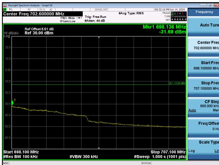
LTE Band 71 / 10MHz / QPSK - RB Size/Offset (25/25)
