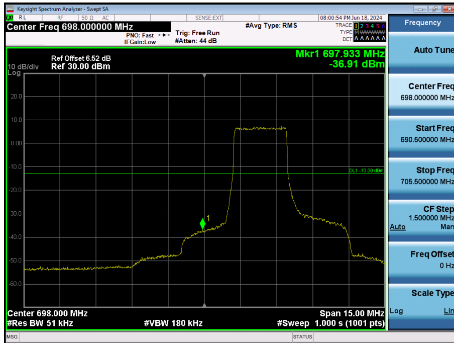
LTE Band 12 / 5MHz / QPSK - RB Size/Offset (12/0)
