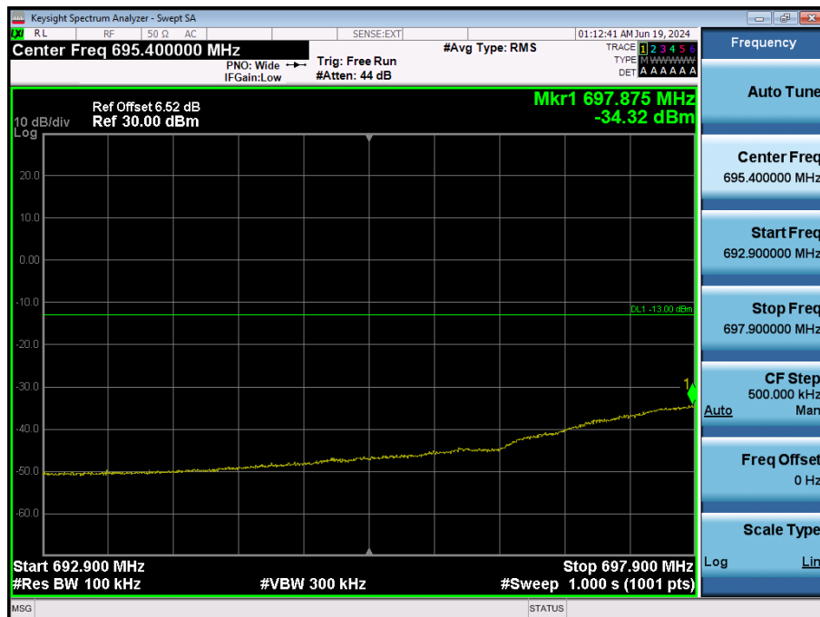
LTE Band 12 / 3MHz / 16QAM - RB Size/Offset (15/0)
