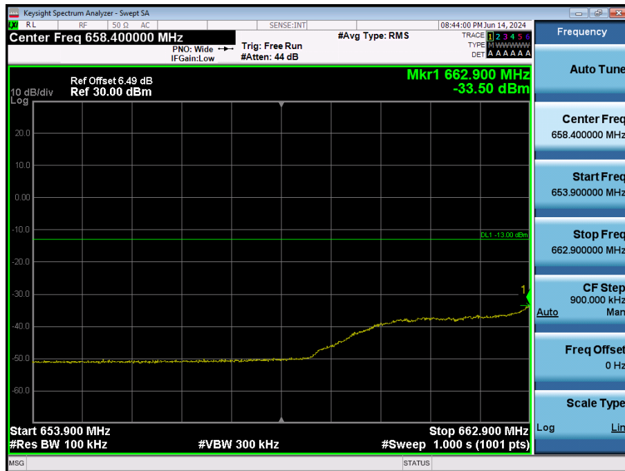
LTE Band 71 / 10MHz / QPSK - RB Size/Offset (25/0)
