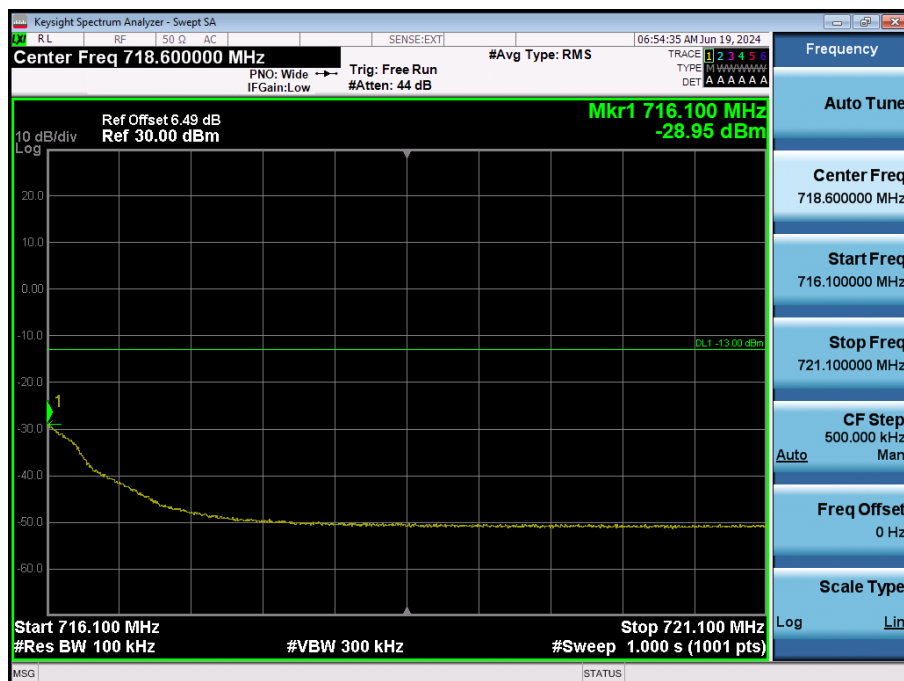
LTE Band 12 / 1.4MHz / 64QAM - RB Size/Offset (3/3)
