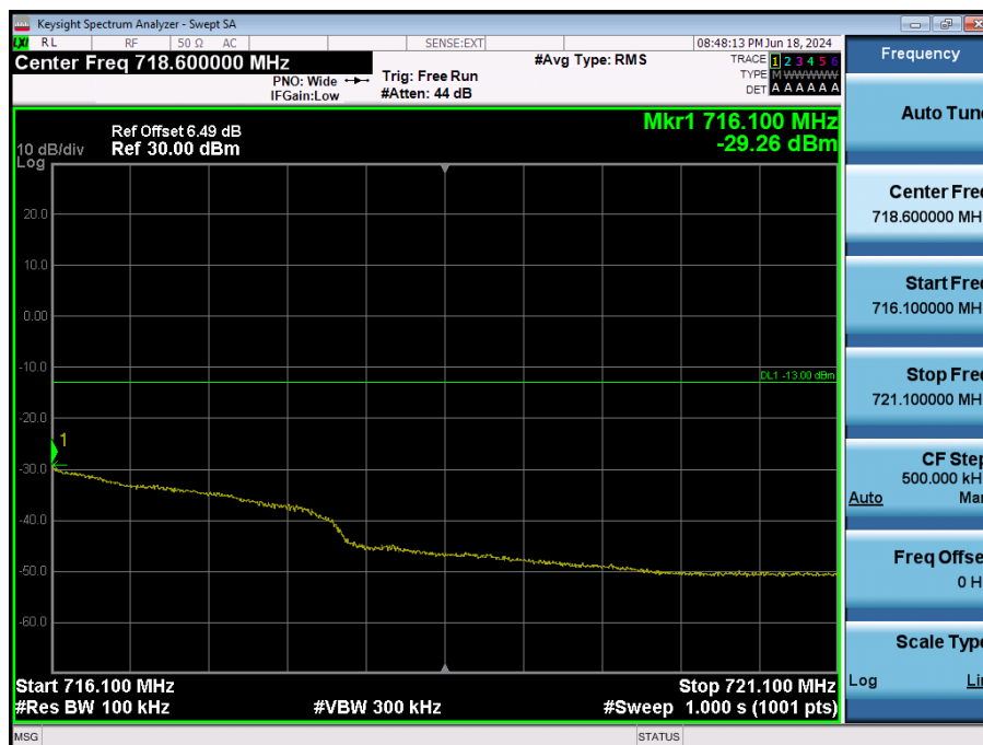
LTE Band 12 / 5MHz / QPSK - RB Size/Offset (12/13)
