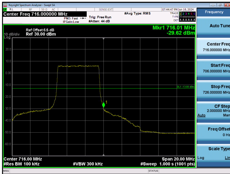
LTE Band 12 / 10MHz / QPSK - RB Size/Offset (25/25)
