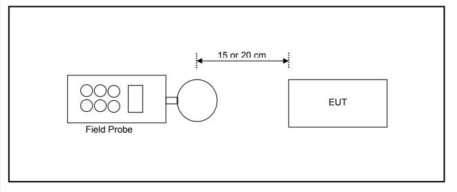
Note: Measurements should be made from all sides and the top of the primary/client pair, with the 15 or 20 cm measured from the center of the probe(s) to the edge of the device.
