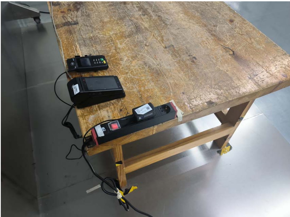
Conducted Emissions Side View
