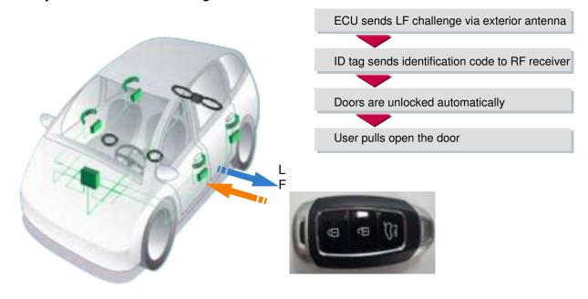
Figure 1: Principle of Communication
