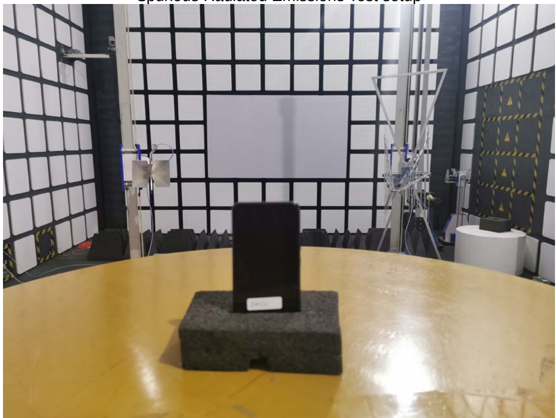
Spurious Radiated Emissions Test setup
