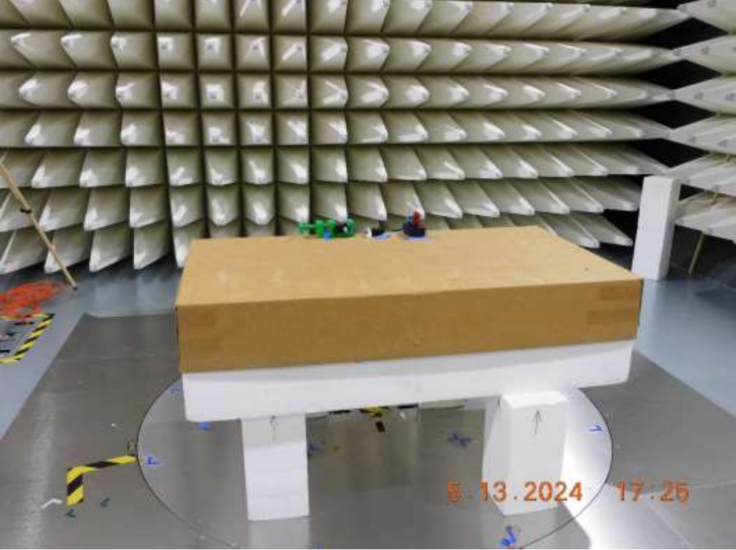
Figure RE30.2: EUT test setup, front view
