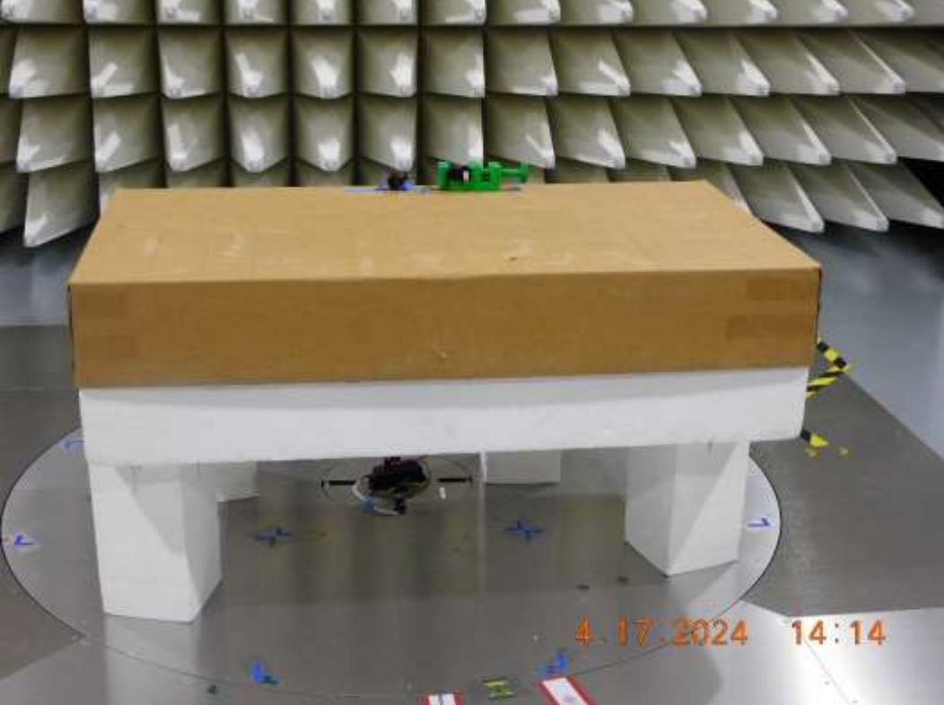
Figure RE25.2: EUT test setup, front view
