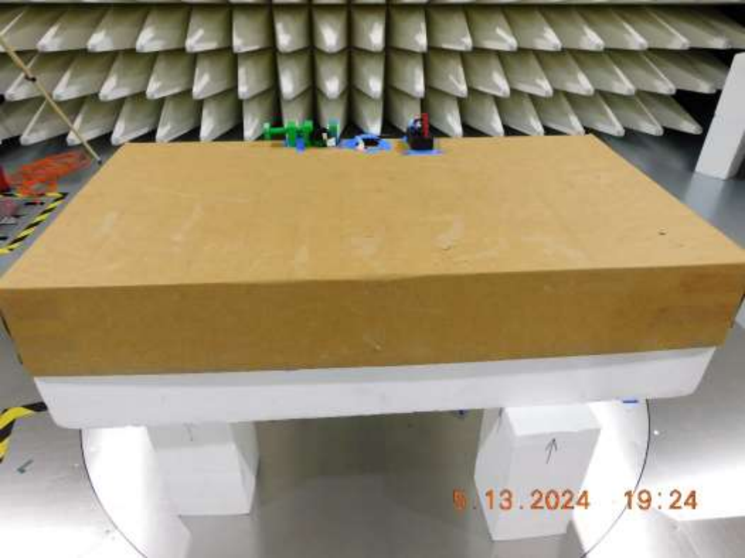
Figure RE31.2: EUT test setup, front view
