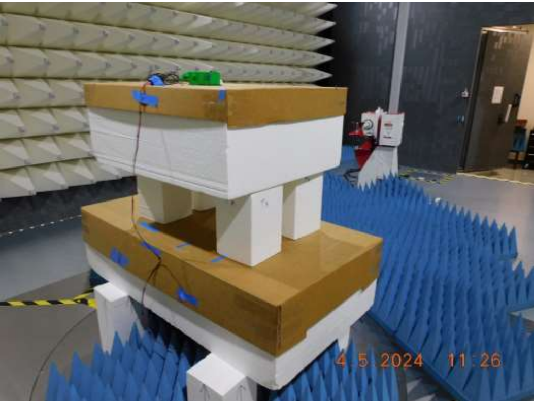
Figure RE05.5: EUT test setup, reverse view
