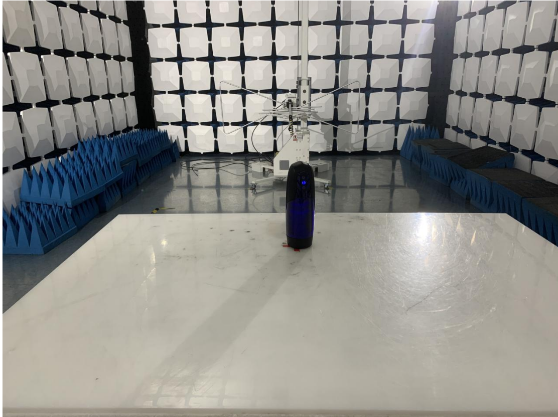
Below 1GHz for radiated emission test setup
