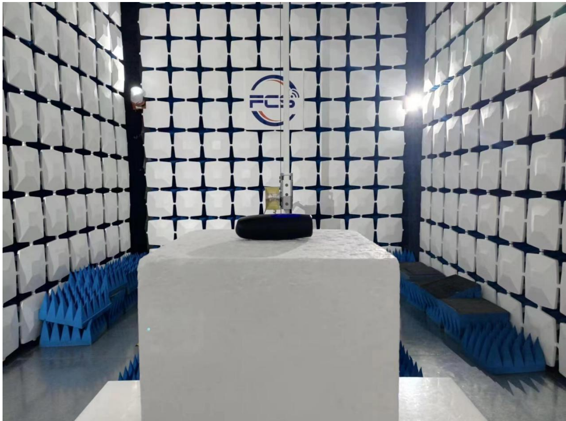
Above 1GHz for radiated emission test setup
