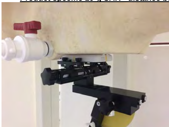
Fig.9 EUT Back side to flat phantom
