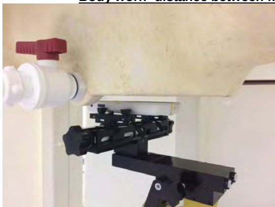
Fig.7 EUT Front side to flat phantom
