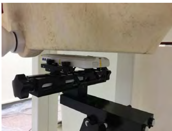
Fig.8 EUT Back side to flat phantom
