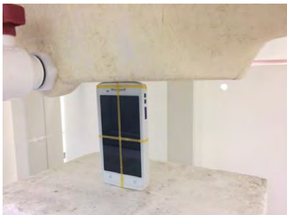
Fig.11 EUT Top side to flat phantom
