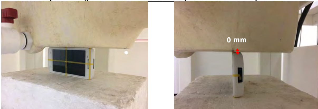
Fig.12 EUT Left side to flat phantom
