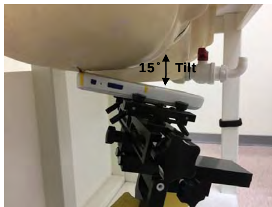
Fig.4 Right Head Section / Ear-Tilt Position(15°)
