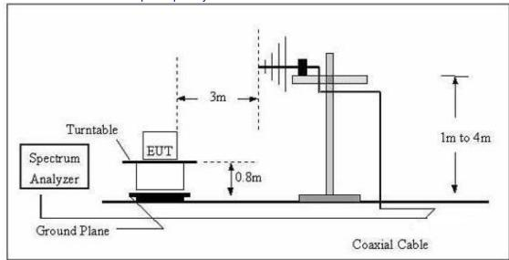
(C) Radiated Emission Test-Up Frequency Above 1GHz
