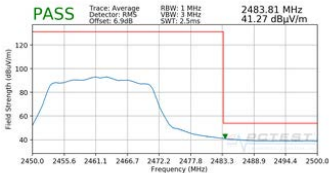
Plot 7-83. Radiated Restricted Band Edge Measurement SISO ANT2 with WCP (Average)
