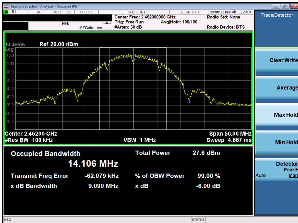
Plot 7-12. 6dB Bandwidth Plot SISO ANT1 (802.11b – Ch. 11)
