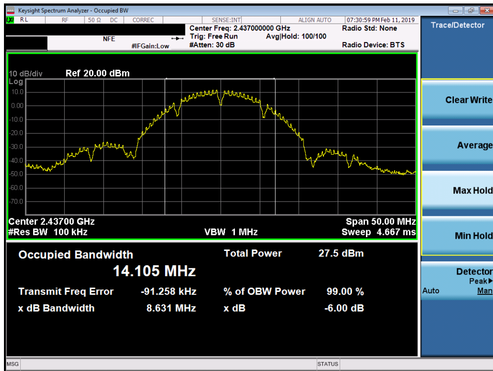
Plot 7-2. 6dB Bandwidth Plot SISO ANT1 (802.11b – Ch. 6)
