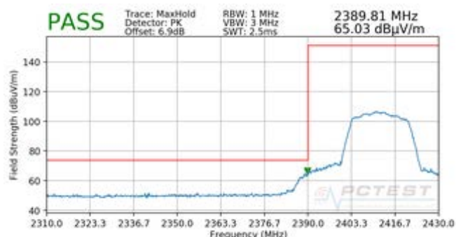
Plot 7-74. Radiated Restricted Lower Band Edge Measurement SISO ANT1 (Peak)
