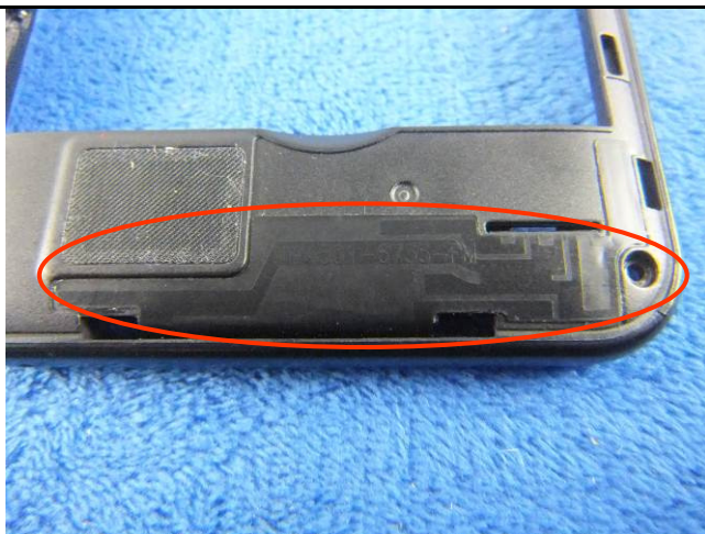
GSM/PCS/UMTS-FDD Antenna View
