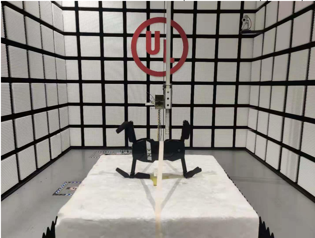
Radiated Disturbance Below 1 GHz and Above 30 MHz (WiFi)
