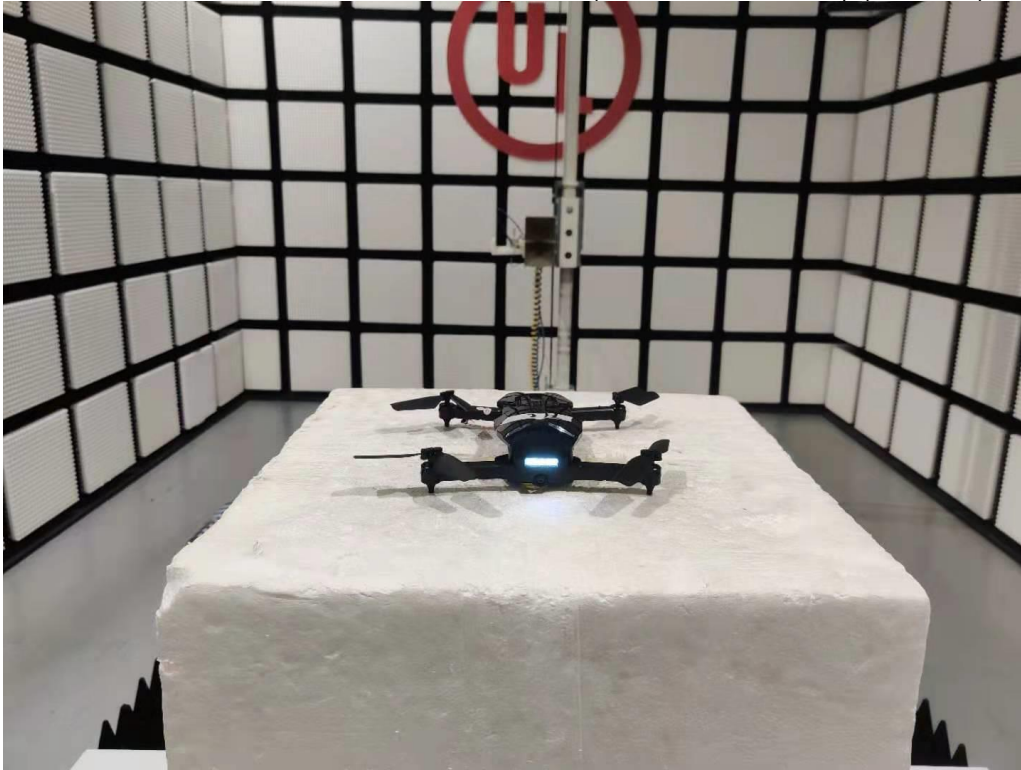
RADIATED RF MEASUREMENT SETUP (Above 1G – X axis) (2.4 GHz)
