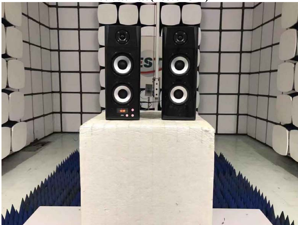
Radiated Test (Above 1GHz)
