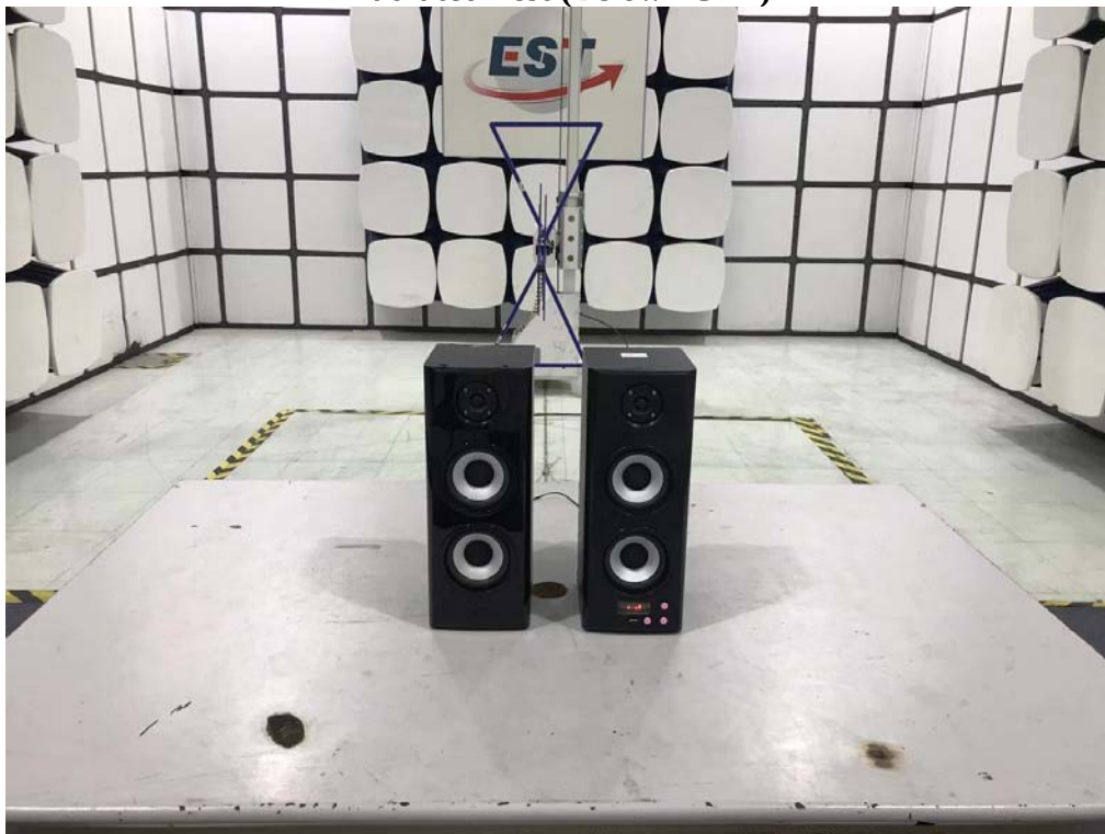
Radiated Test (Below 1GHz)
