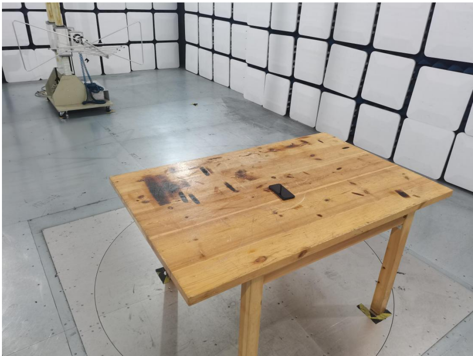
Photo of Radiation Emission Test
