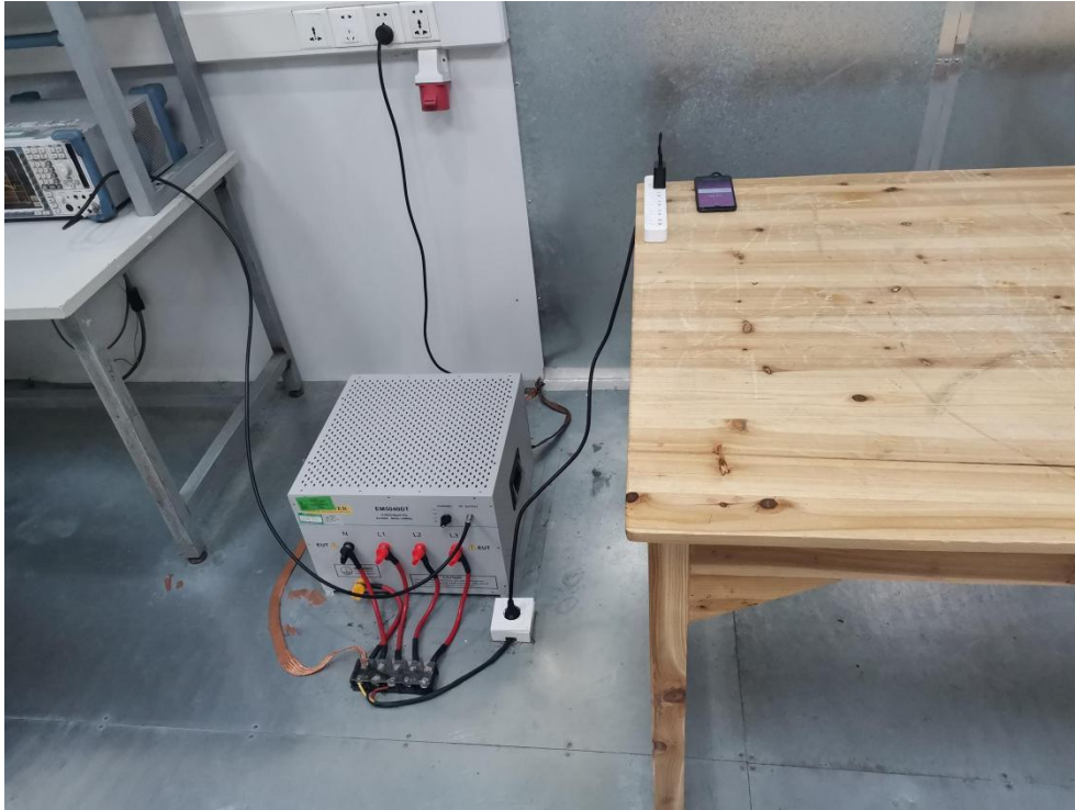
Photo of Conducted Emission Measurement
