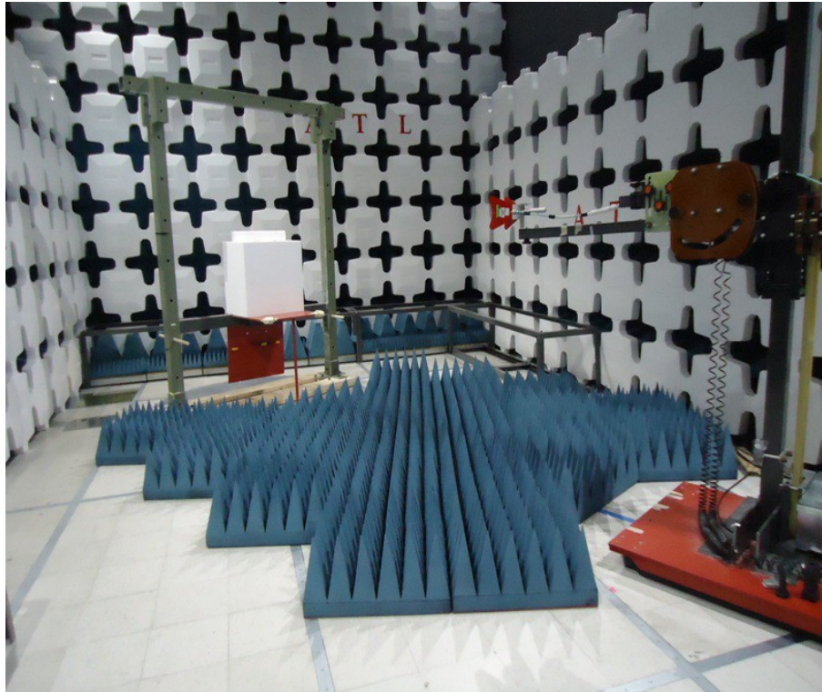
Figure 3.2 - Test Facility (Setup for 1GHz – 18GHz)
