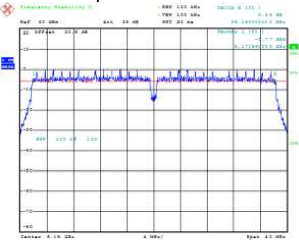
Figure 8-16: 6 dB Bandwidth Secondary, 802.11ac, Channel 36, MCS0 Mbps
