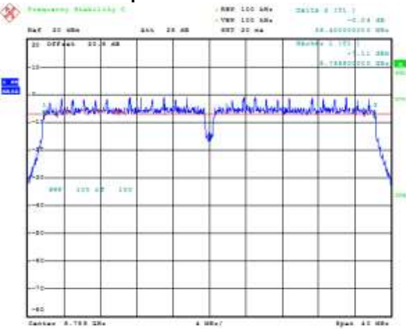
Figure 8-20: 6 dB Bandwidth Secondary, 802.11ac, Channel 149, MCS0 Mbps
