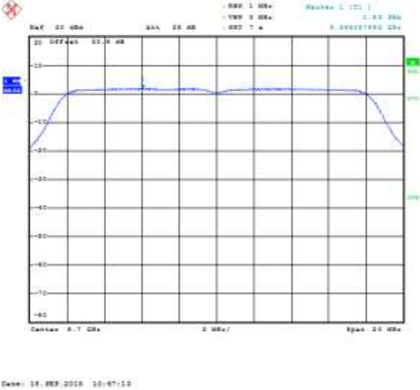
Figure 7-76: Peak Power Spectral Density SISO Secondary, 802.11a, Channel 140, 6 Mbps
