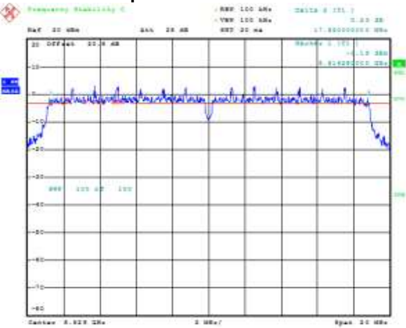
Figure 8-10: 6 dB Bandwidth Secondary, 802.11ac, Channel 149, MCS0 Mbps
