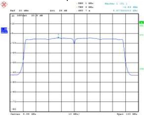
Figure 8-104: Peak Power Spectral Density SISO Secondary, 802.11ac, Channel 155, MCS0 Mbps
