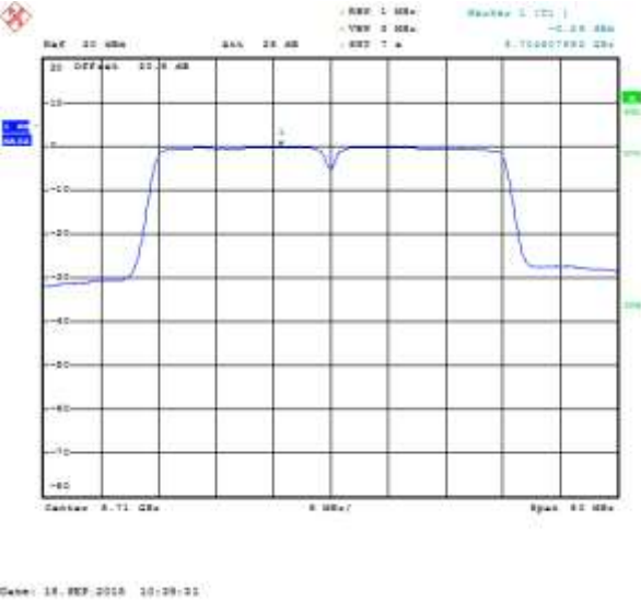
Figure 7-113: Peak Power Spectral Density SISO Secondary, 802.11n, Channel 140, MCS 0
