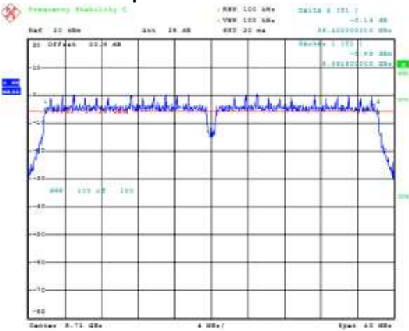
Figure 8-19: 6 dB Bandwidth Secondary, 802.11ac, Channel 140, MCS0 Mbps
