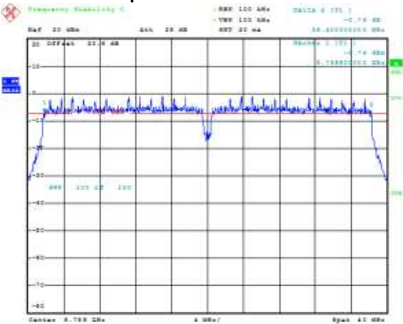
Figure 8-15: 6 dB Bandwidth Primary, 802.11ac, Channel 149, MCS0 Mbps
