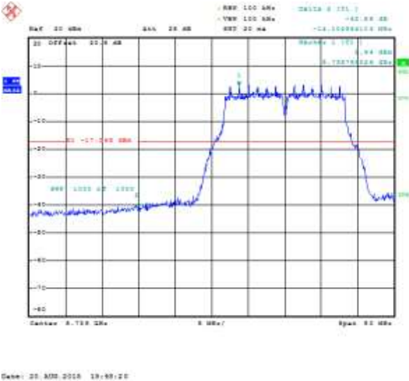
Figure 7-36: Band Edge Compliance Primary, 802.11a, Channel 149, 6 Mbps
