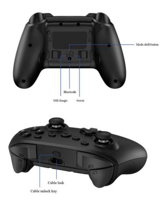
Note: Left Joystick can be L3 when vertical press; Right Joystick can be R3 when vertical press; Power indicators or channel indicators are LED1, LED2, LED3, LED4 from left to right.
