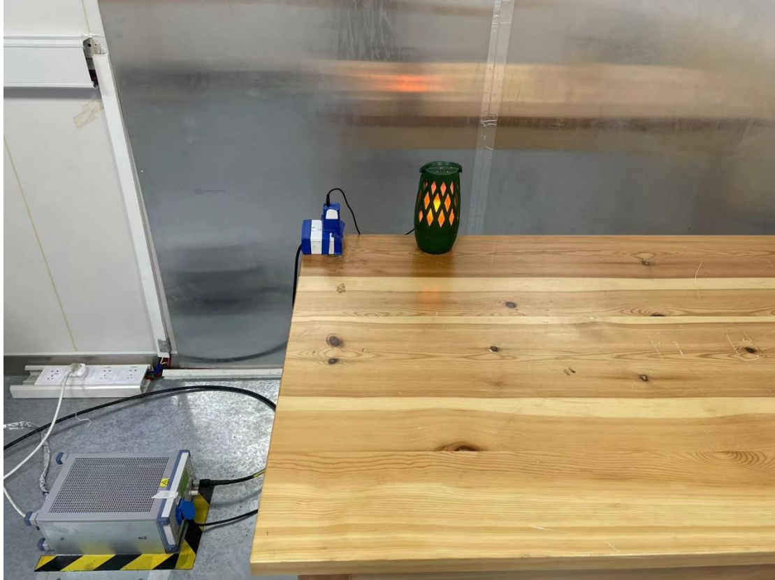
Conducted emission test setup
