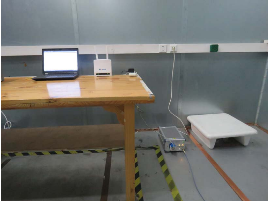
Picture 3 Conducted Emission Test Setup
