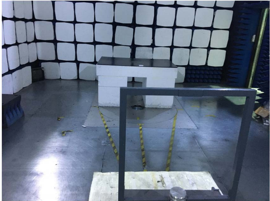
Radiation Emission Test Setup (Below 30MHz)
