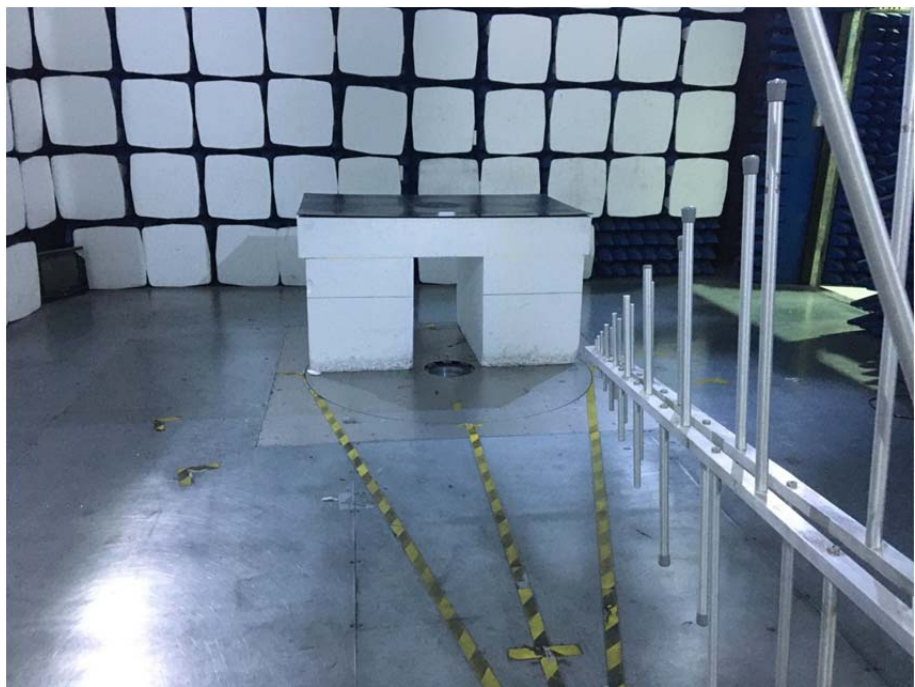
Radiation Emission Test Setup (30MHz to 1GHz)
