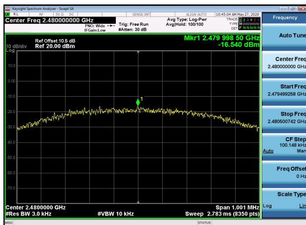
Power spectral density: 2480MHz
