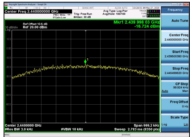
Power spectral density: 2440MHz
