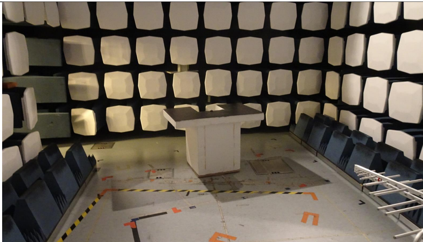
Picture 8, Radiated Spurious Emissions, common setup, TX and RX 30 - 1000 MHz
