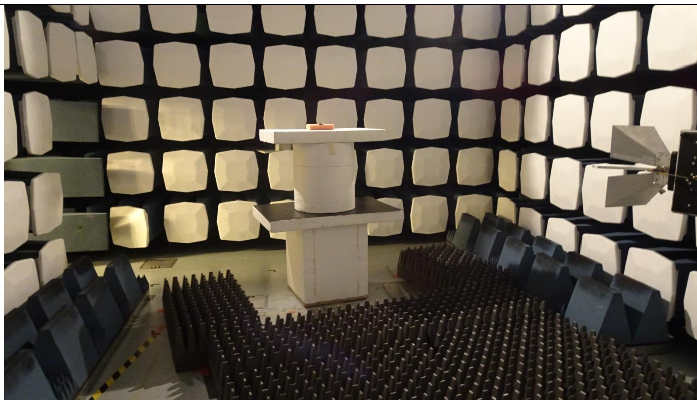
Picture 9, Radiated Spurious Emissions, common setup, TX, 1 - 26 GHz
