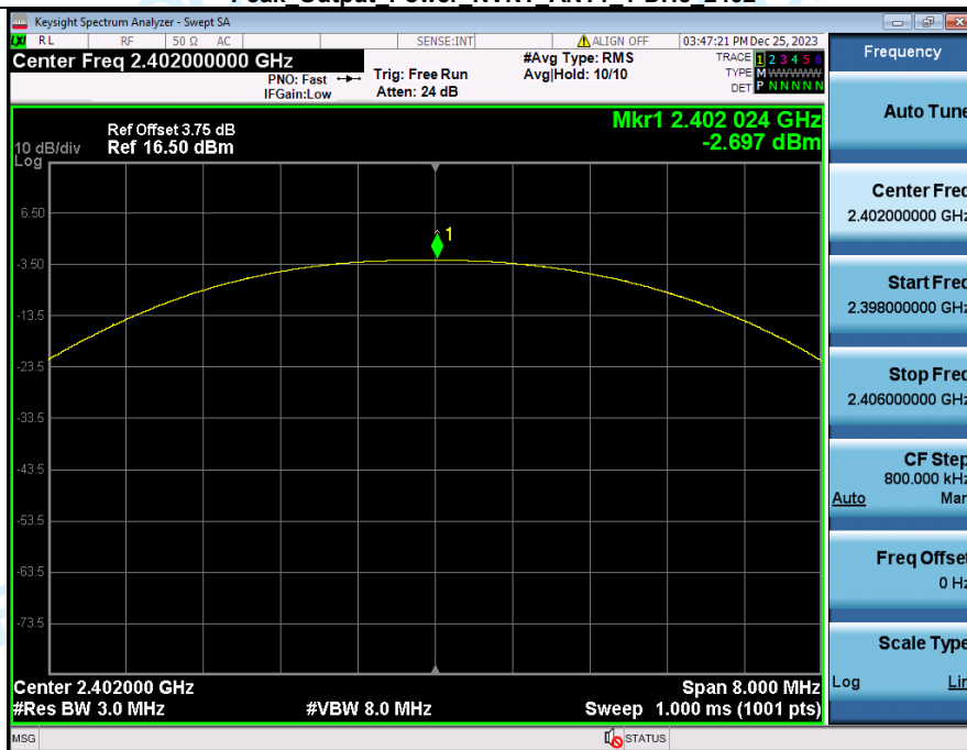
Peak Output Power NVNT ANT1 1-DH5 2402
