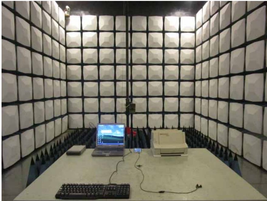
Radiated Emission –Front View (Above 1 GHz)
