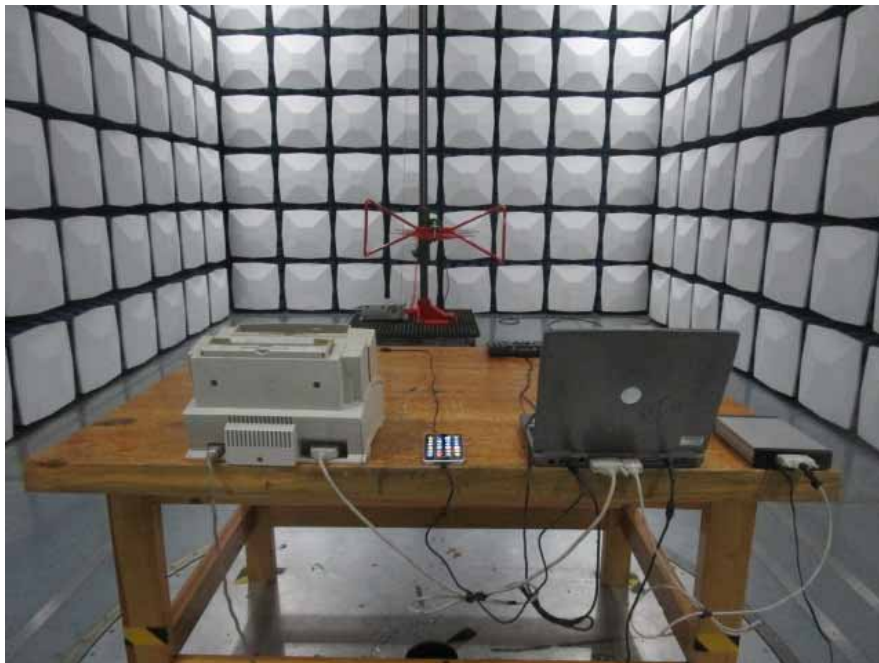
Radiated Emissions –Rear View (Below 1GHz)
