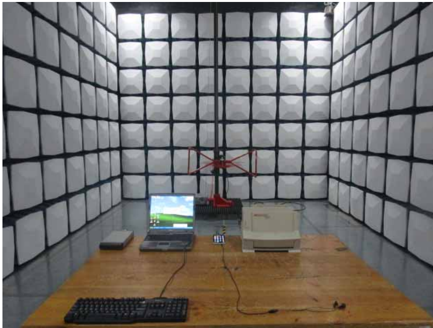
Radiated Emissions –Front View (Below 1GHz)
