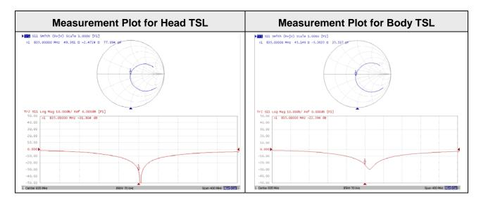
The impedance is within 5 ohm of prior calibration.
